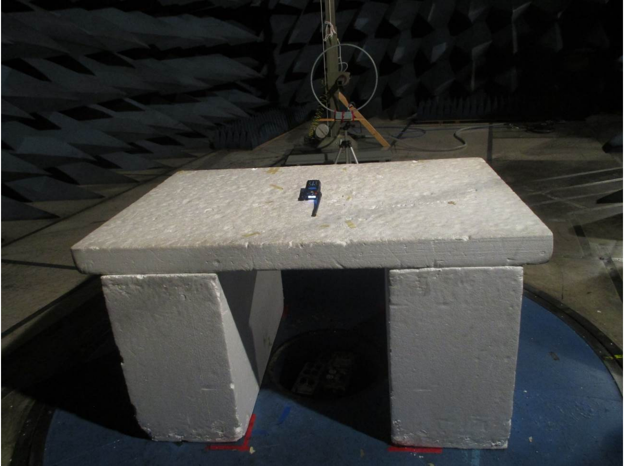
Figure 4: Radiated Emissions – Back View – 9 kHz – 30 MHz
