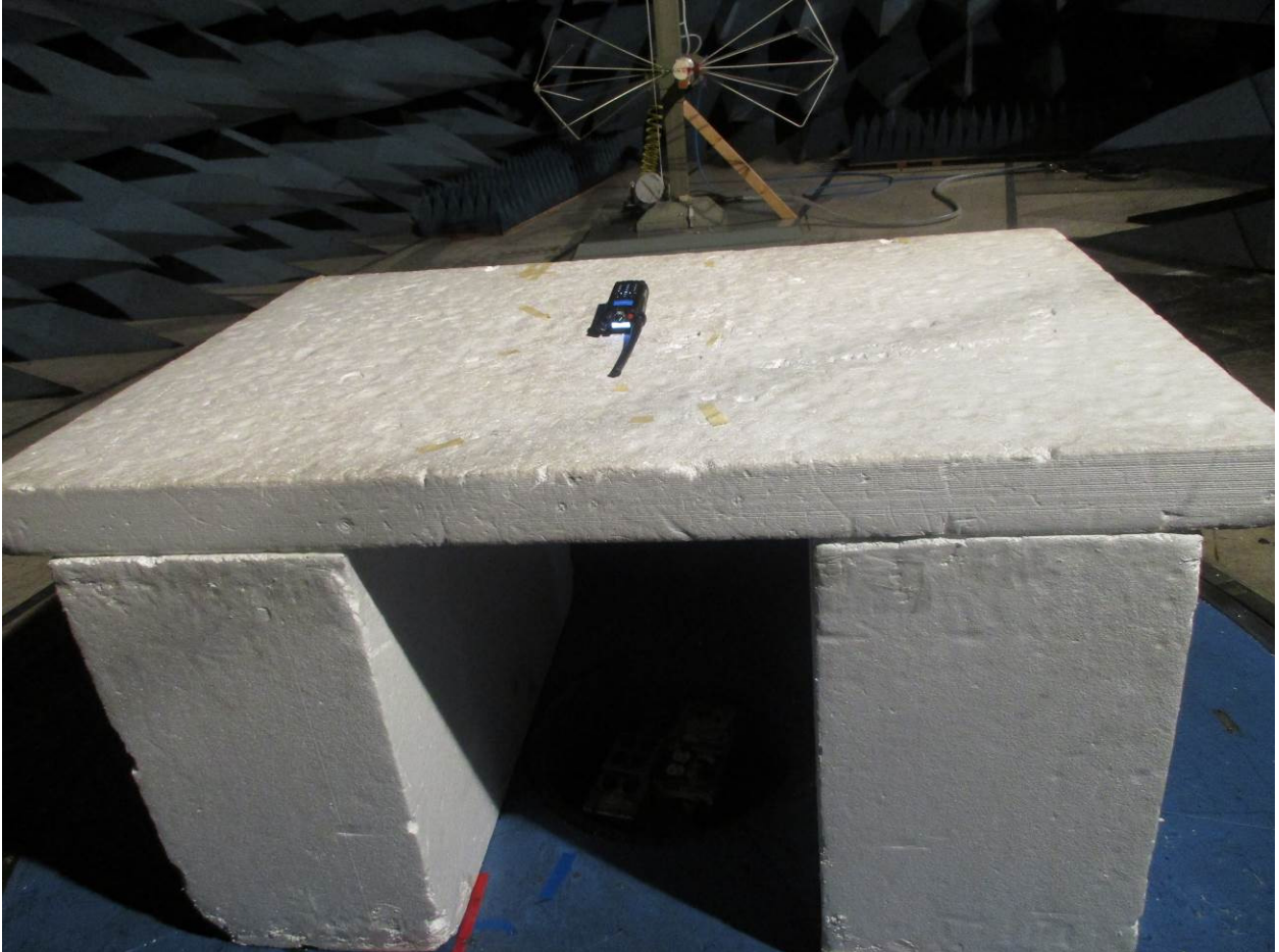
Figure 5: Radiated Emissions – Back View – 30 MHz – 200 MHz
