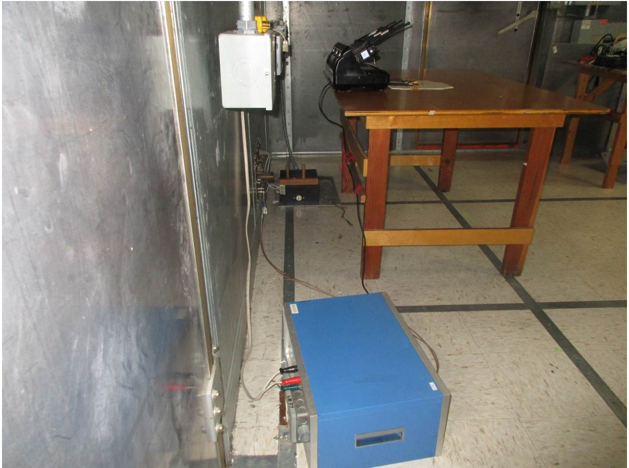
Figure 11: Power Line Conducted Emissions – Side View
