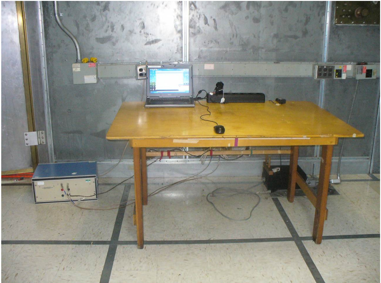
Figure 7: Power Line Conducted Emissions – Front View
