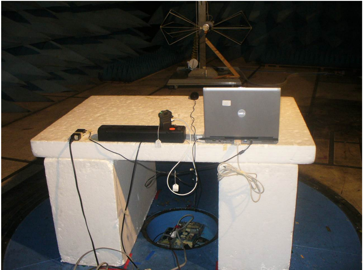
Figure 3: Radiated Emissions – Back View 30 MHz - 200 MHz
