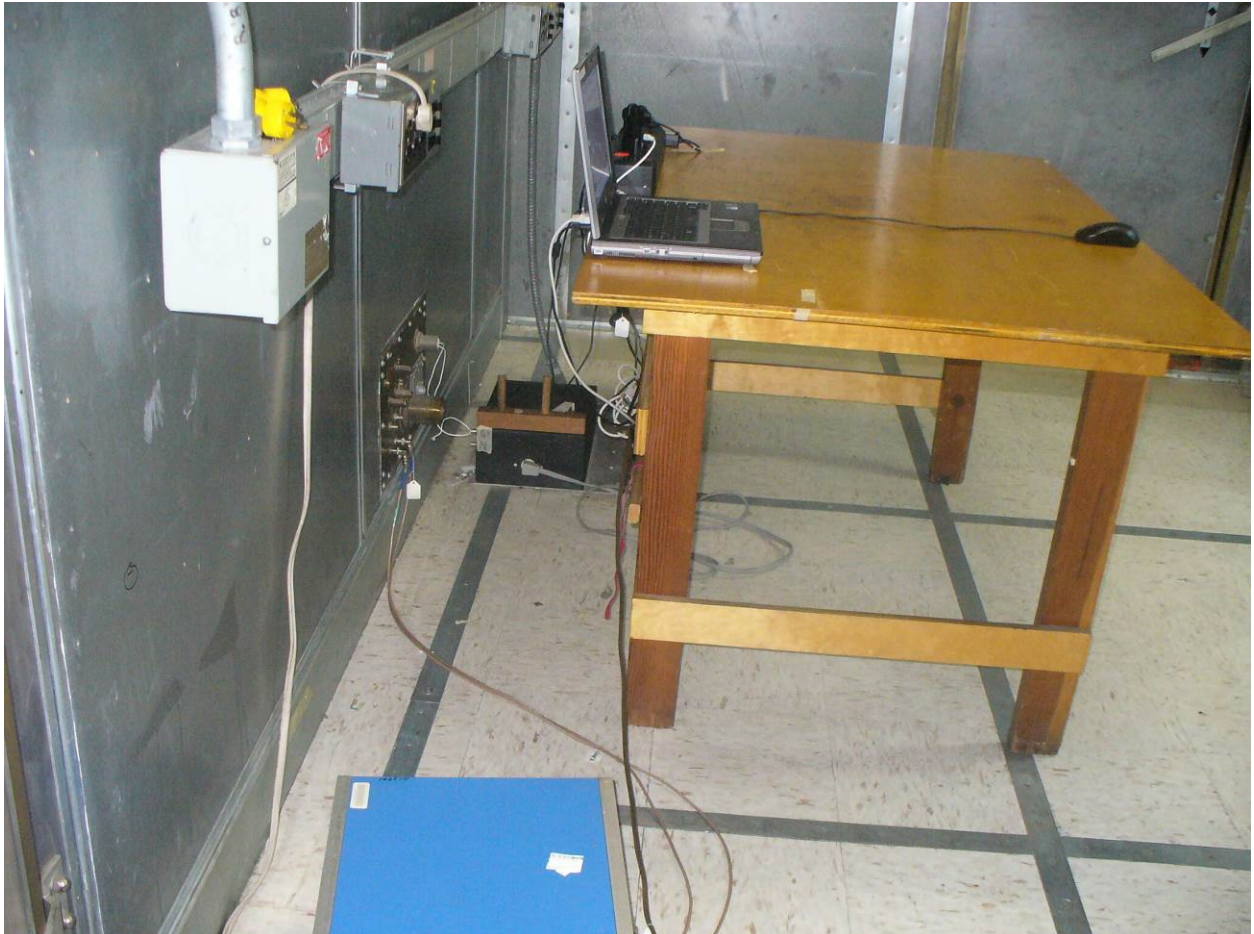
Figure 8: Power Line Conducted Emissions – Side View
