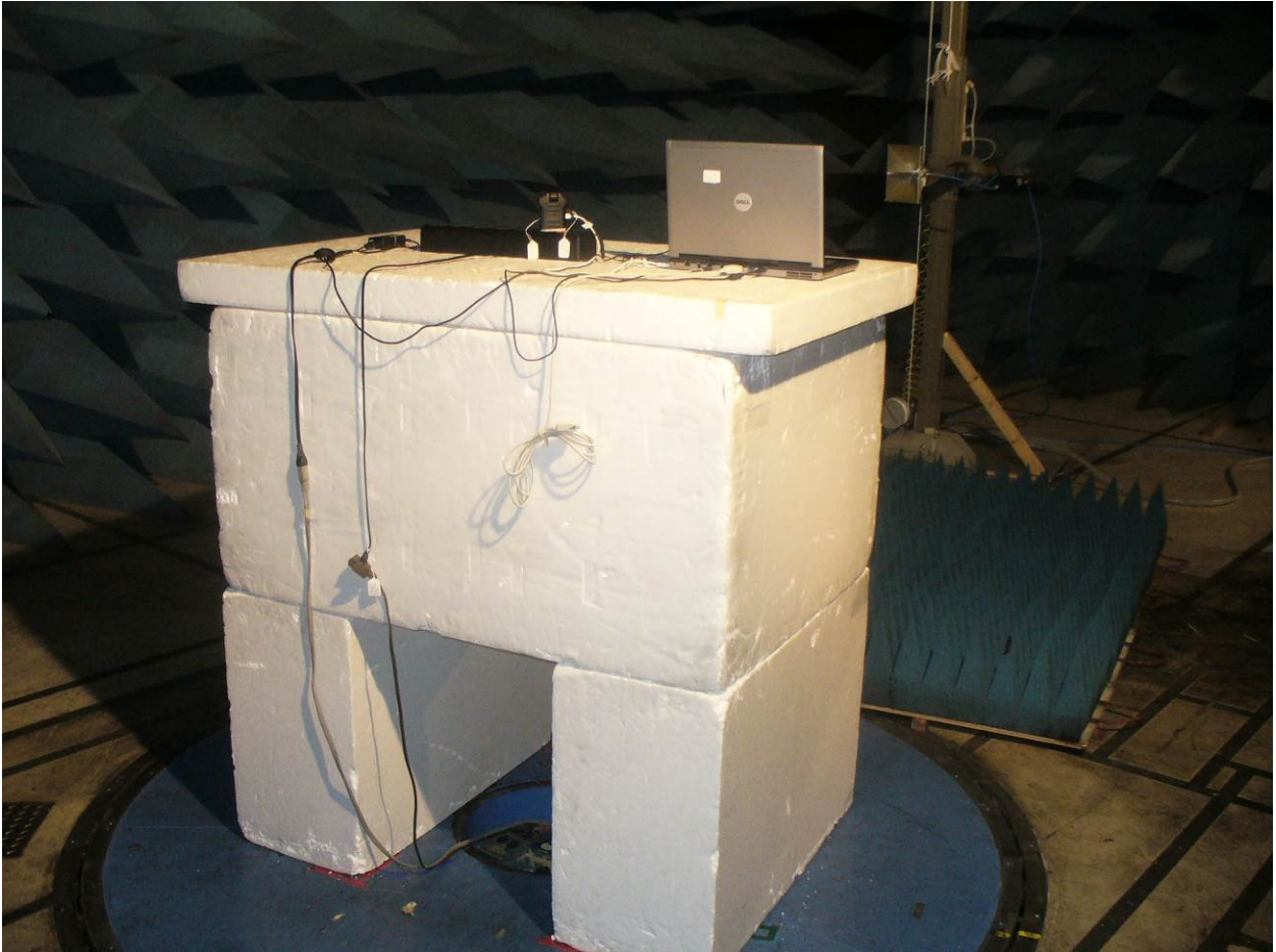
Figure 6: Radiated Emissions – Back View above 1 GHz
