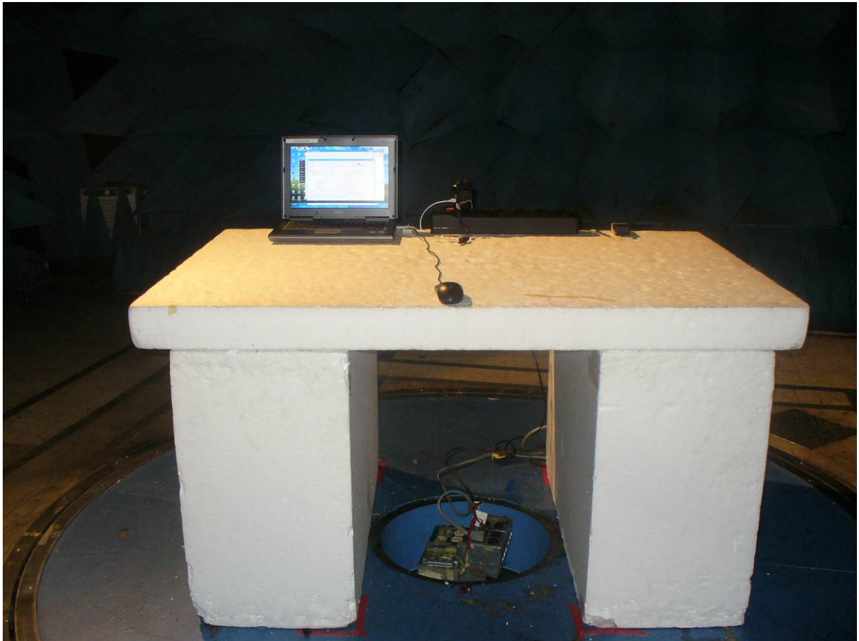
Figure 1: Radiated Emissions – Front View below 1 GHz
