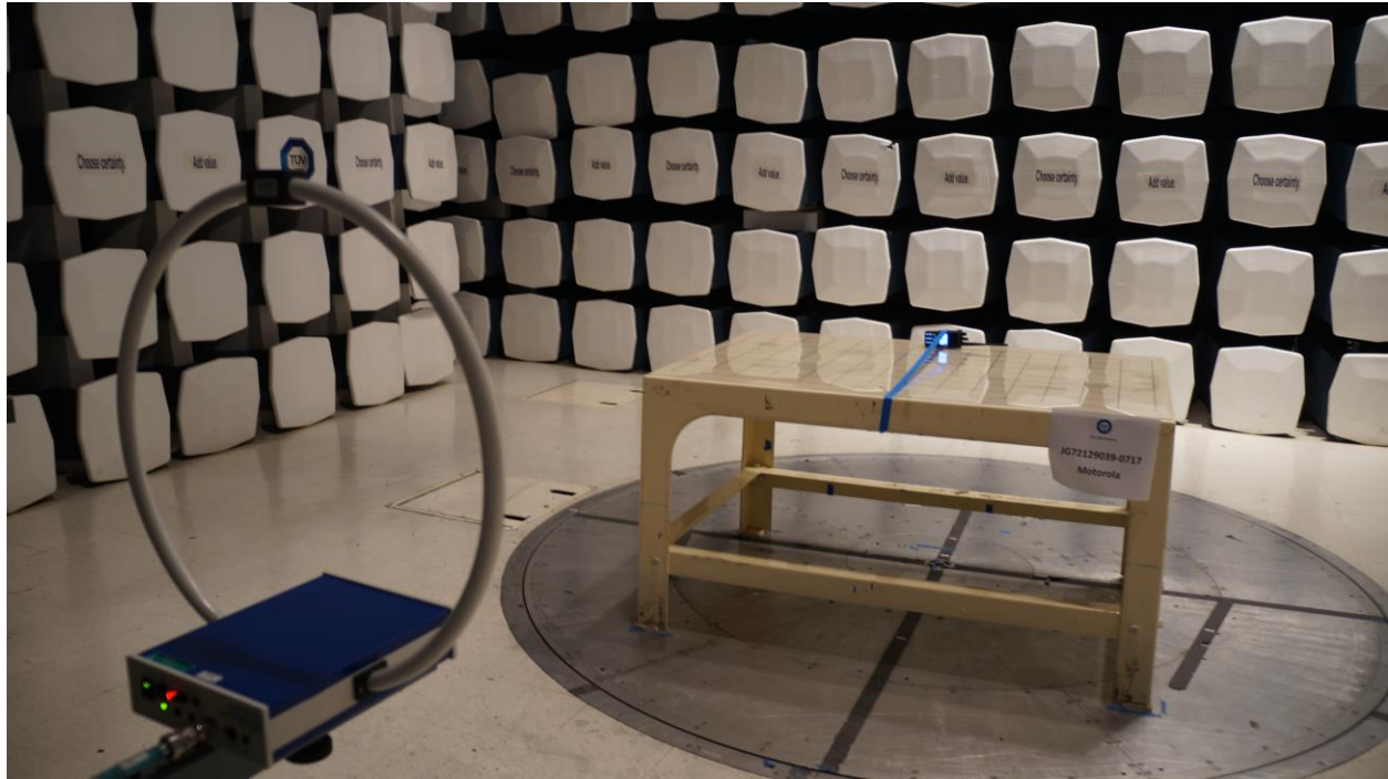
Radiated Emissions Test Setup (Below 30 MHz - Front)
