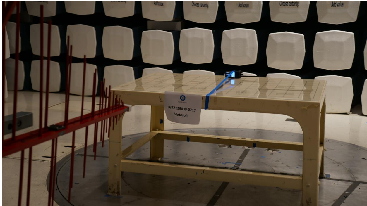
Radiated Emissions Test Setup (Below 1000 MHz - Front)
