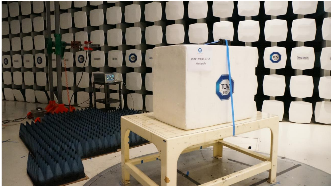
Radiated Emissions Test Setup (Above 1000 MHz - Back)
