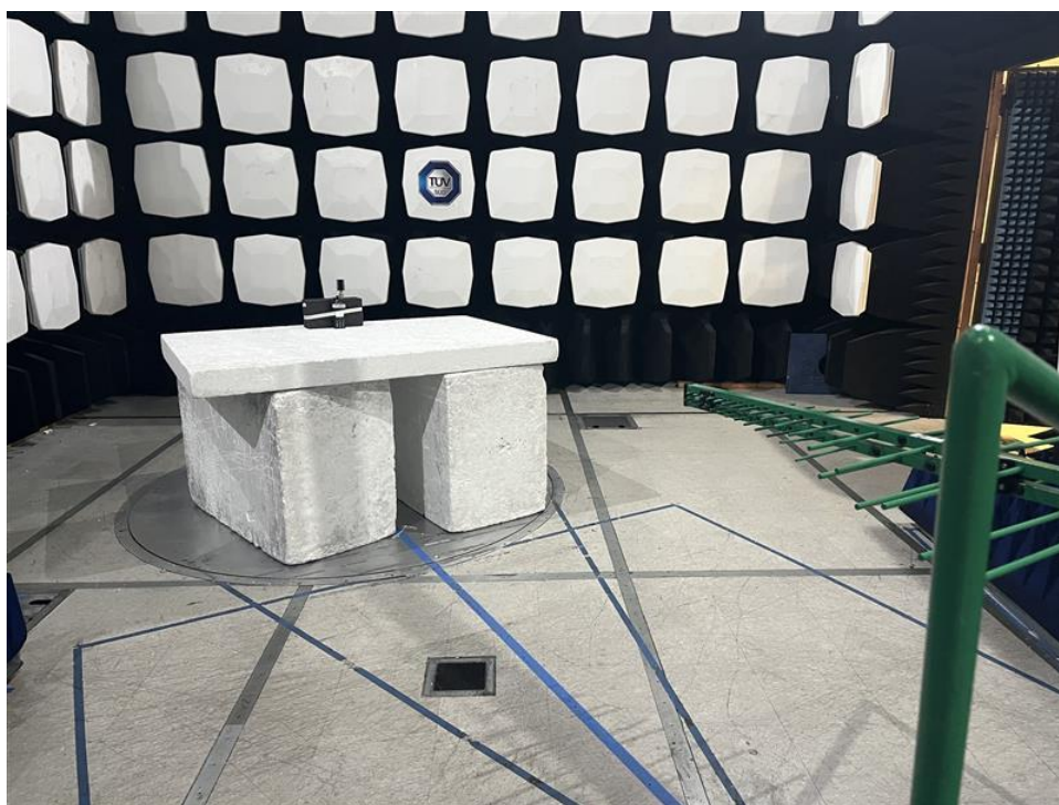
Figure A-4: Test Setup – Radiated Emissions < 1GHz
