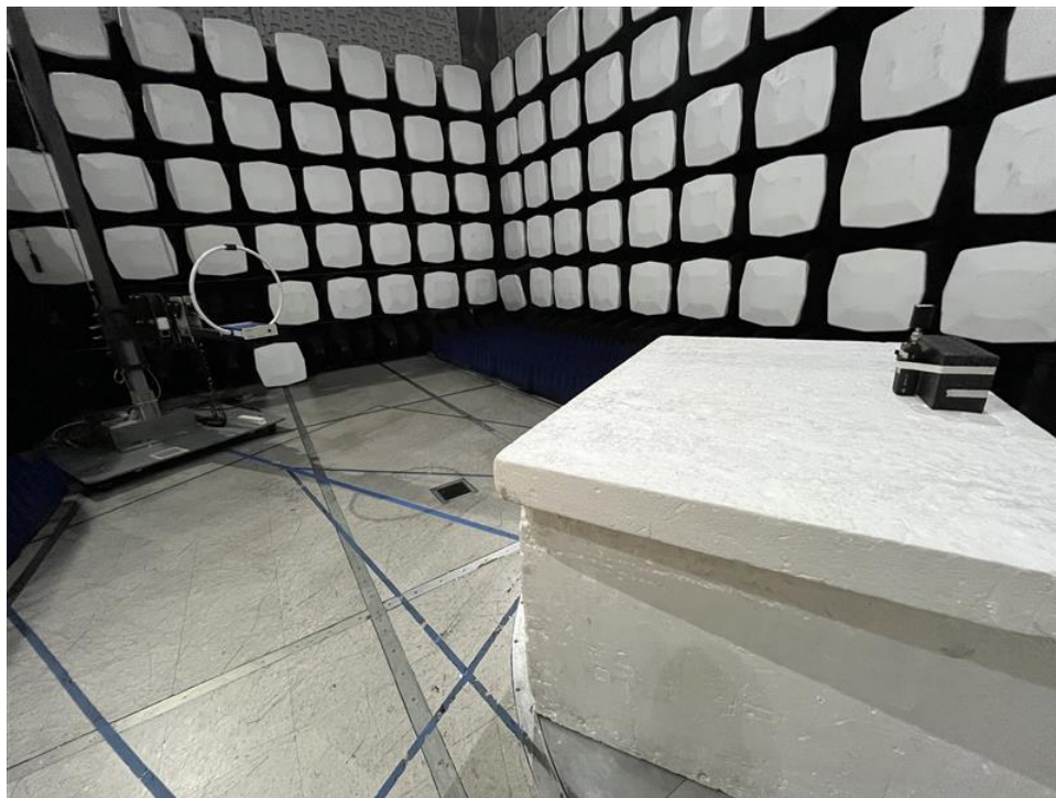
Figure A-1: Test Setup – Radiated Emissions <30 MHz
