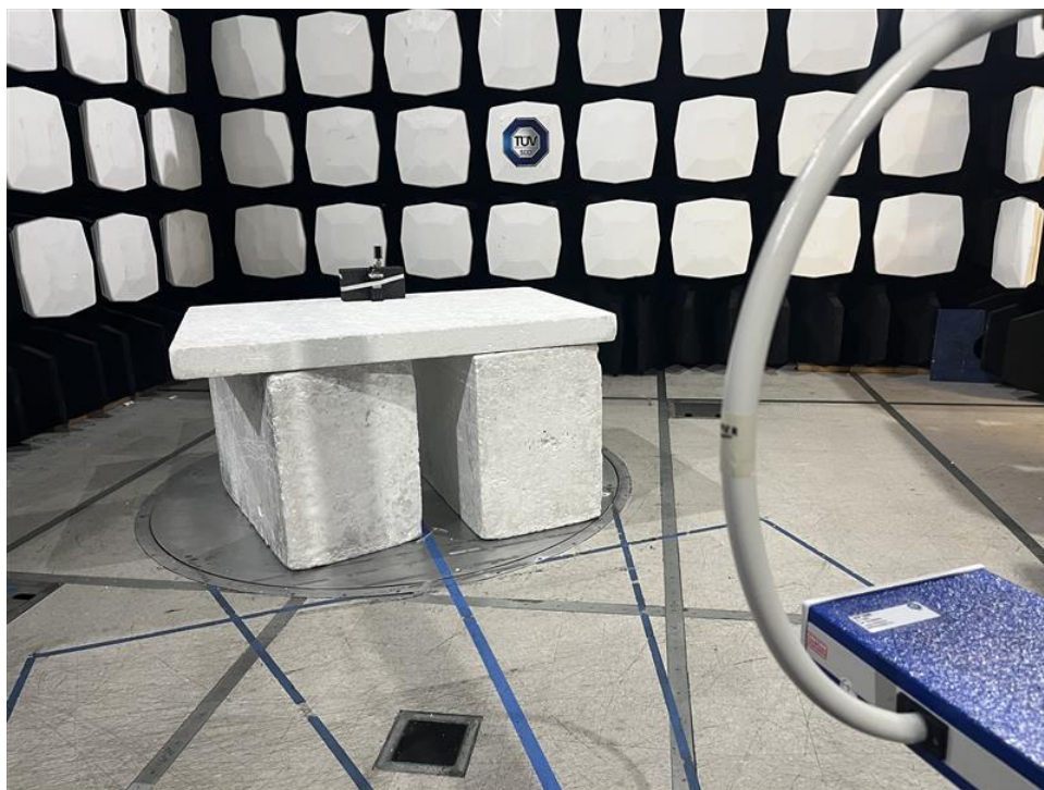
Figure A-2: Test Setup – Radiated Emissions < 30 MHz
