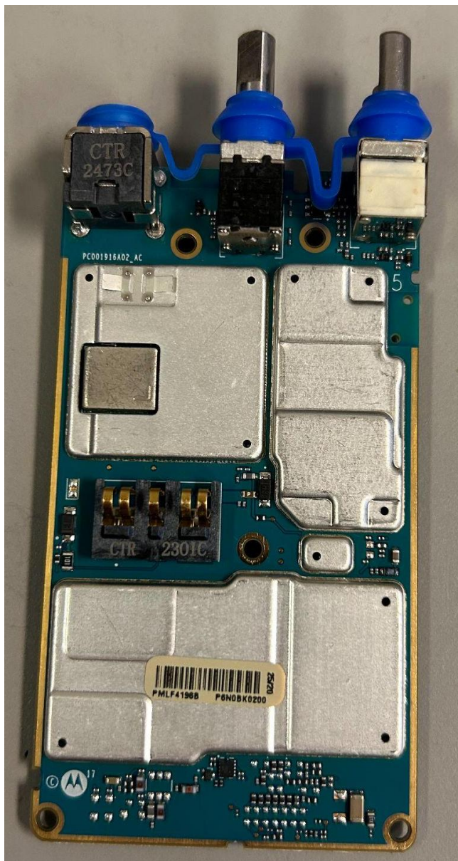
RF board with Shields (Bottom) H92WCF9PW6AN (APX 900)
