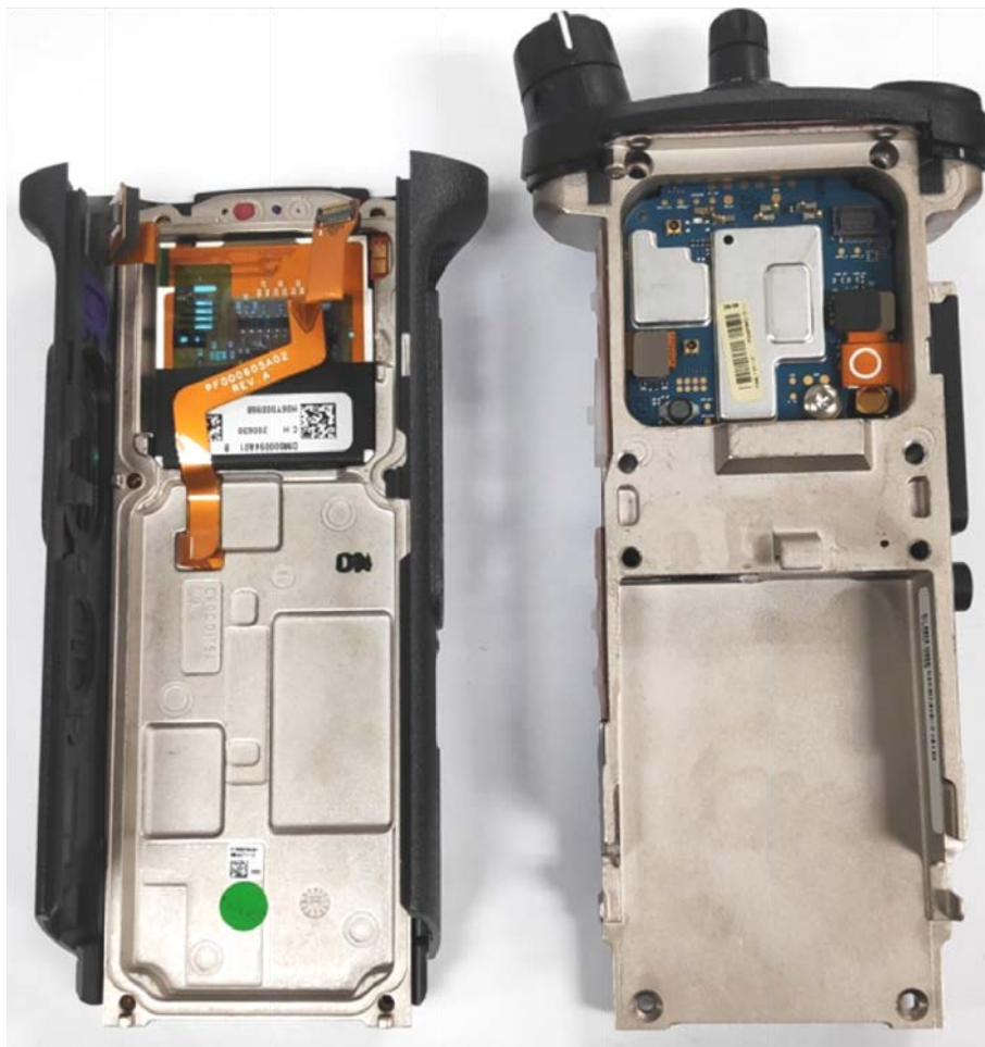
Expansion board with chassis and housing of APX8000H Model 2.5 BLK/BRN (Back side)
