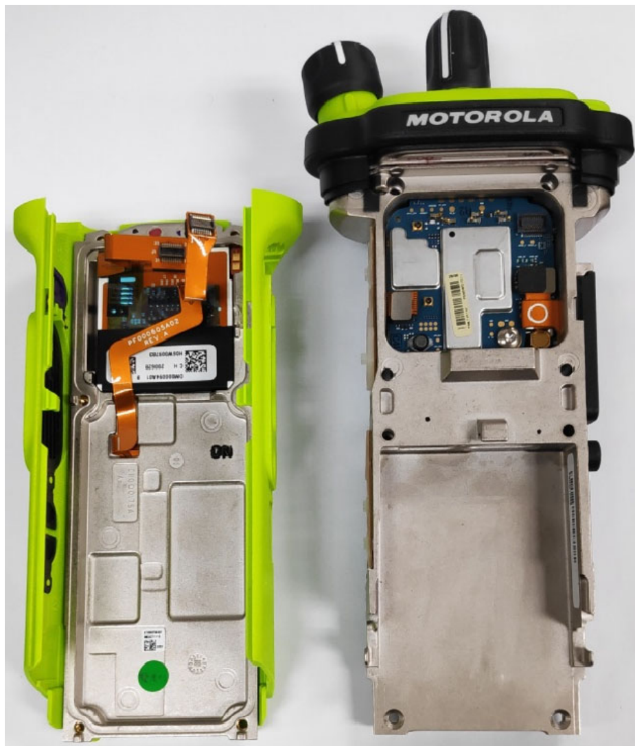
Expansion board with chassis and housing of APX8000HXE Model 3.5 (Back side)
