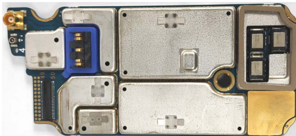
RF board with Shields (Bottom) (APX8000H/ APX8000HXE)
