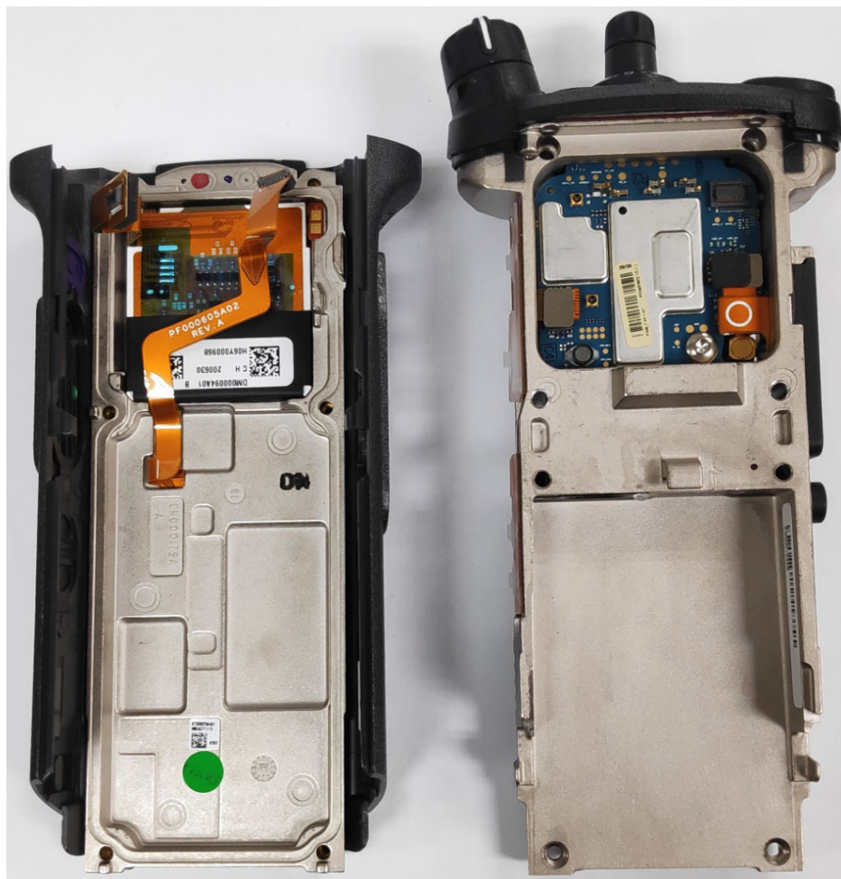
Expansion board with chassis and housing of APX8000H Model 3.5 BLK/BRN (Back side)
