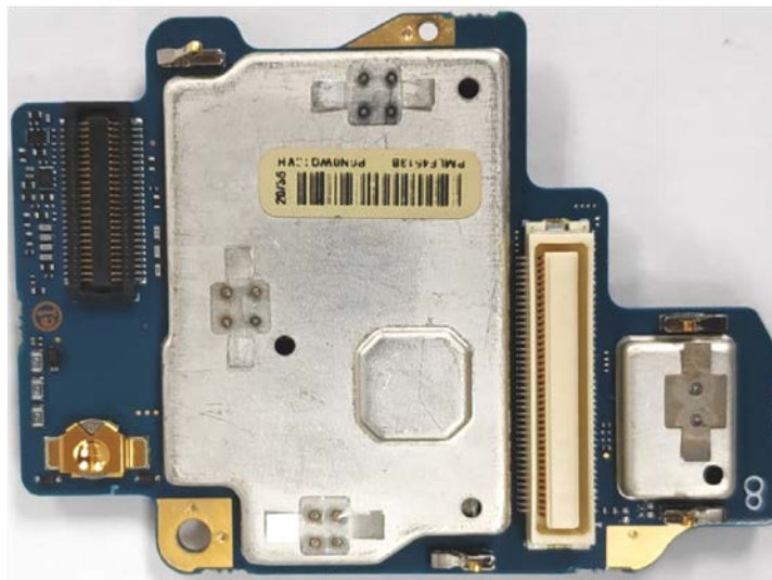
Vocon board with shields (Bottom) (APX8000H/ APX8000HXE)
