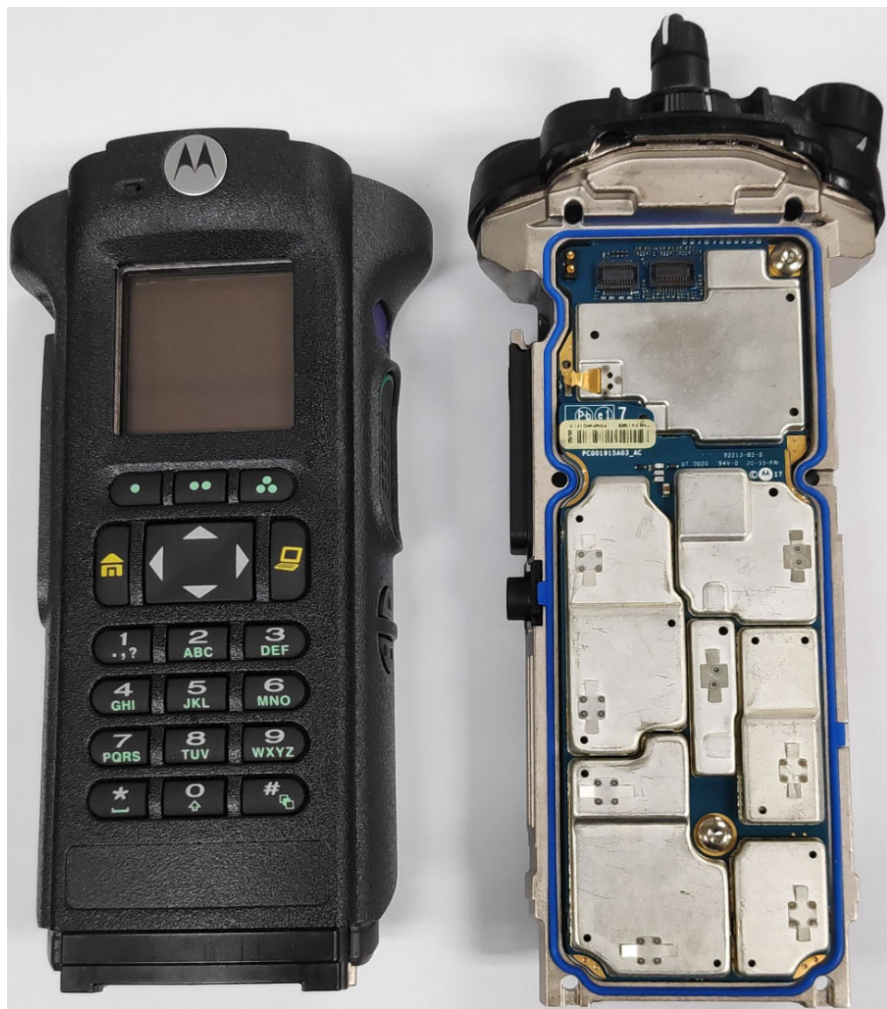
RF and Vocon boards with chassis and housing of APX8000H Model 3.5 BLK/BRN (Front side)
