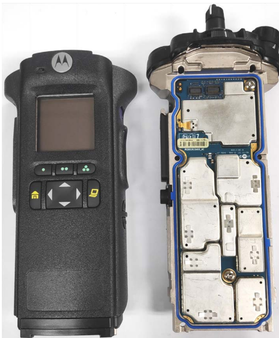
RF and Vocon boards with chassis and housing of APX8000H Model 2.5 BLK/BRN (Front side)
