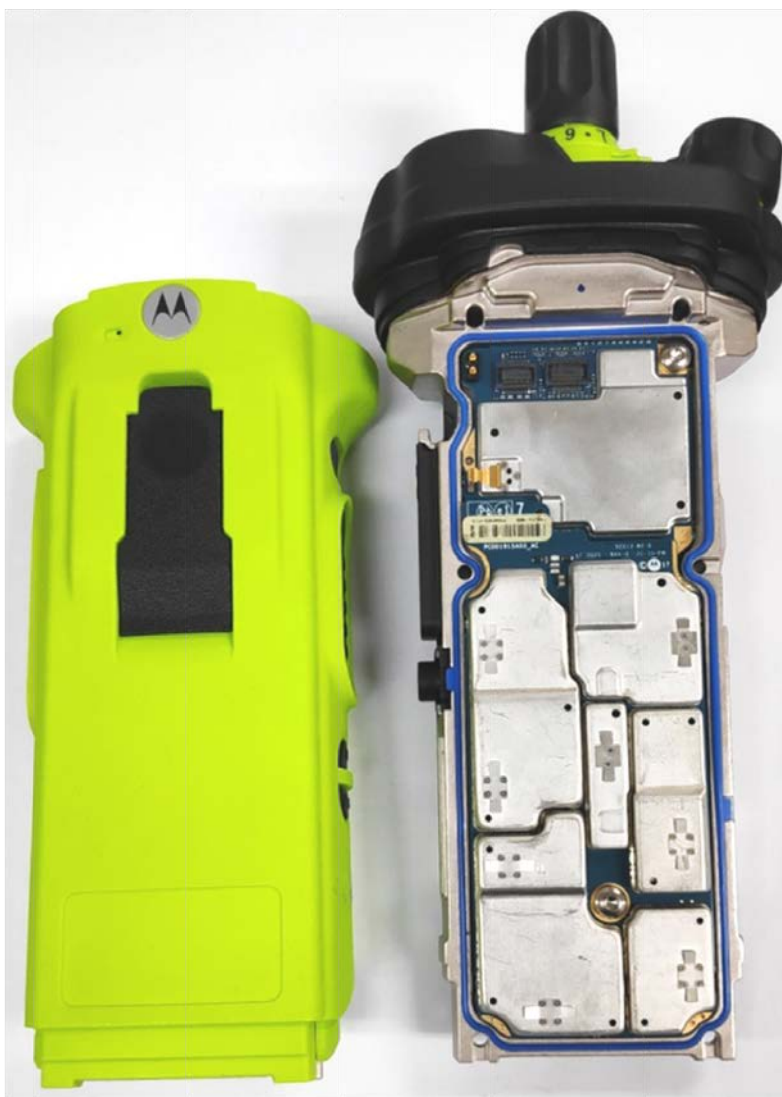
RF and Vocon boards with chassis and housing of APX8000HXE Model 1.5 (Front side)
