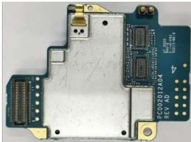
Vocon board with shields (Top) (APX8000H/8000HXE)
