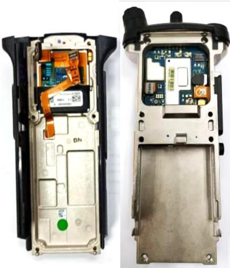
Expansion board with chassis and housing of APX8000H Model 3.5 BLK/BRN (Back side)
