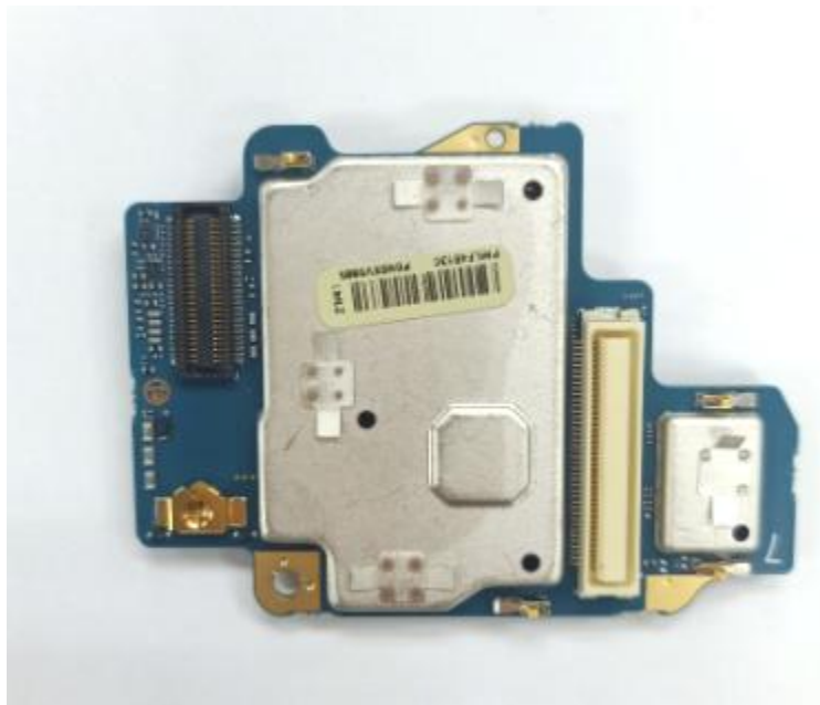
Vocon board with shields (Bottom) (APX8000H/8000HXE)
