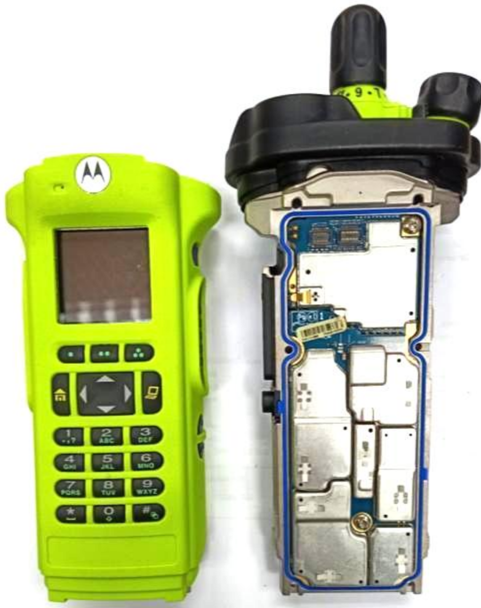
RF and Vocon boards with chassis and housing of APX8000HXE Model 3.5 (Front side)
