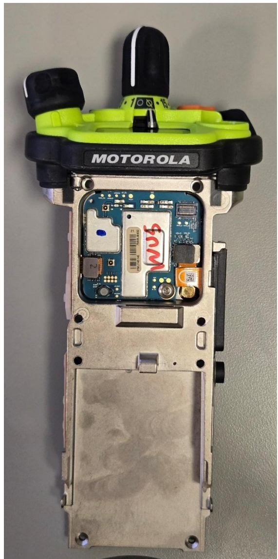
Expansion board with chassis and housing of APX8000HXE Model 3.5 (Back side)
