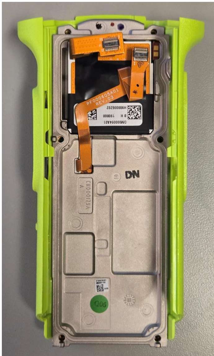
Expansion board with chassis and housing of APX8000HXE Model 3.5 (Back side)
