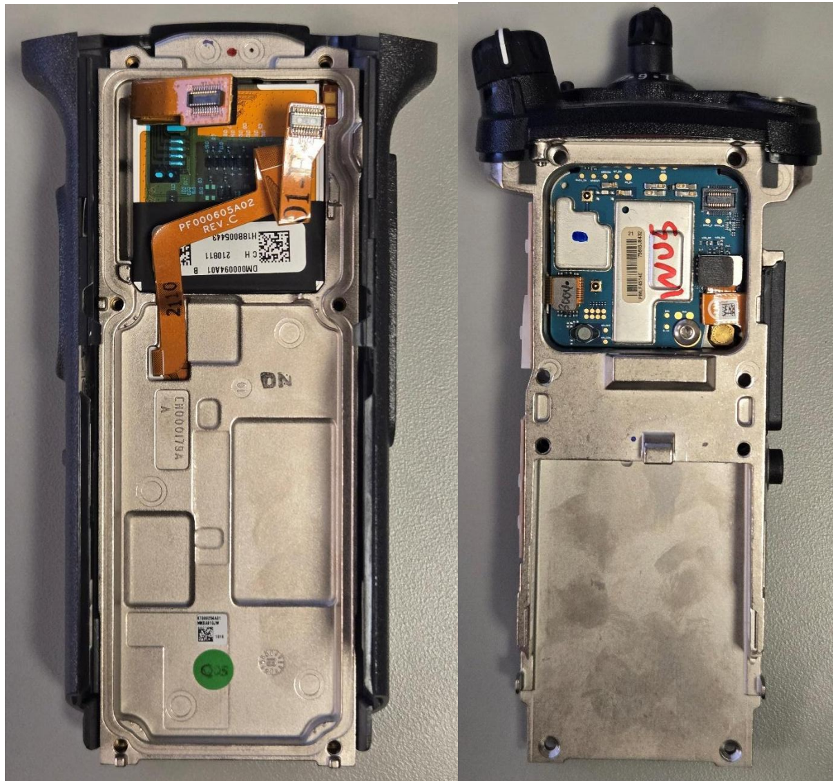
Expansion board with chassis and housing of APX8000H Model 2.5 BLK/BRN (Back side)
