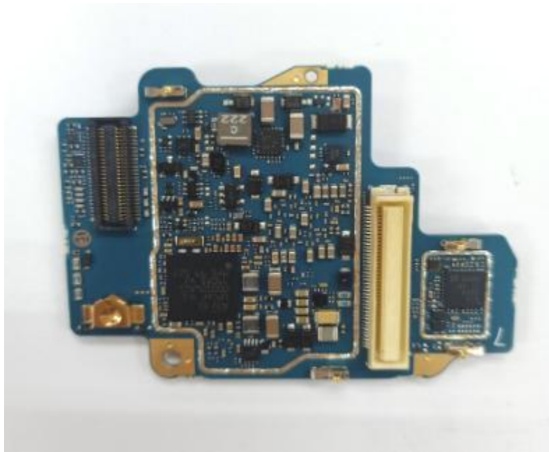
Vocon board without shields (Bottom) (APX8000H/8000HXE)
