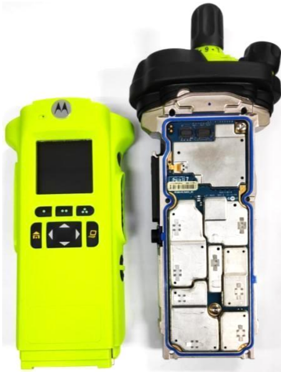
RF and Vocon boards with chassis and housing of APX8000HXE Model 2.5 (Front side)
