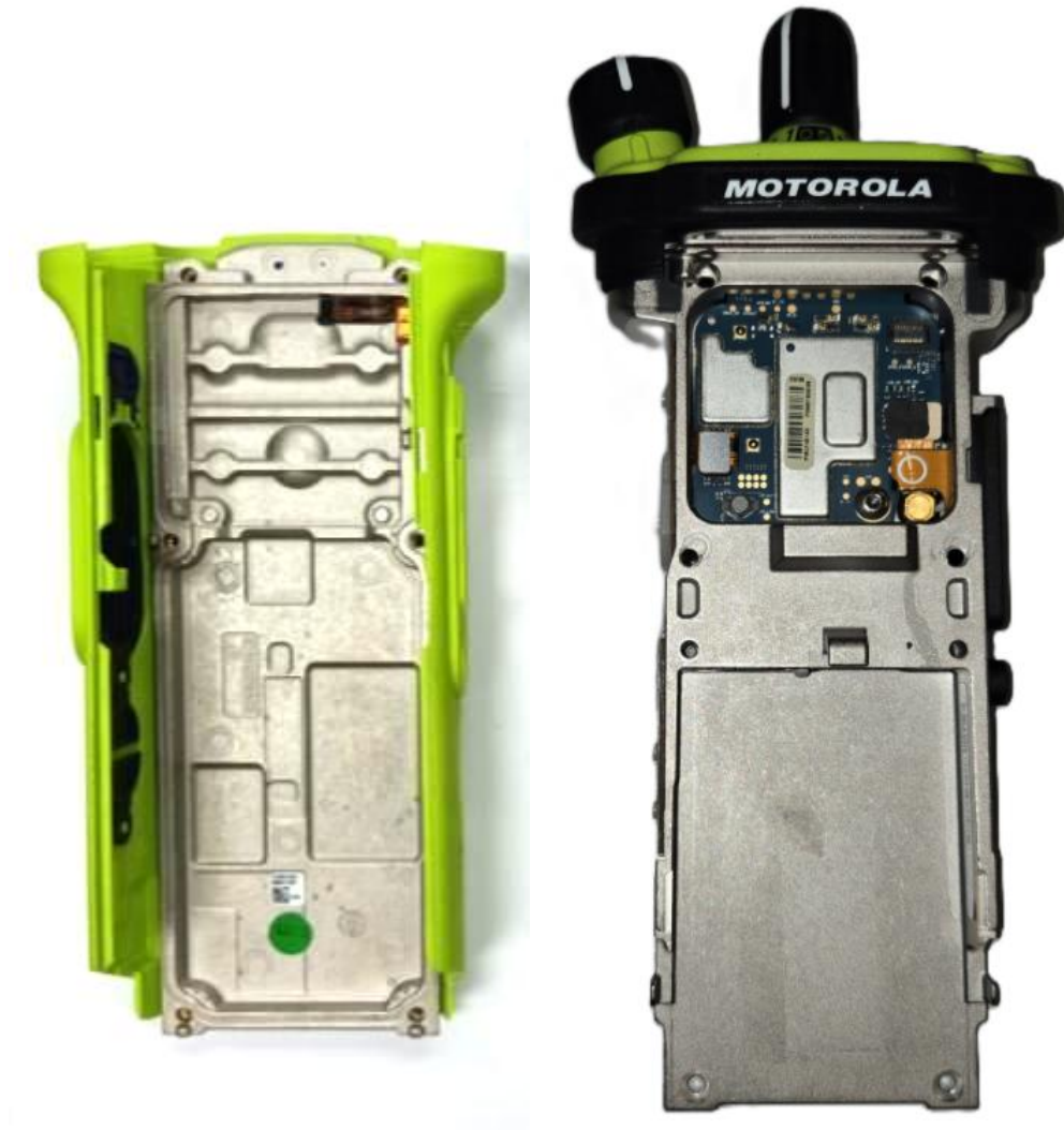
Expansion board with chassis and housing of APX8000HXE Model 1.5 (Back side)
