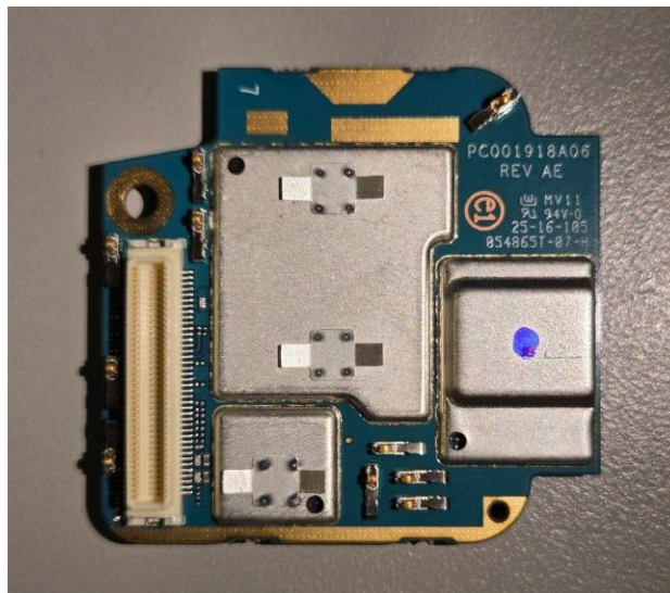
Expansion board with shields (Bottom) (APX8000/8000XE)
