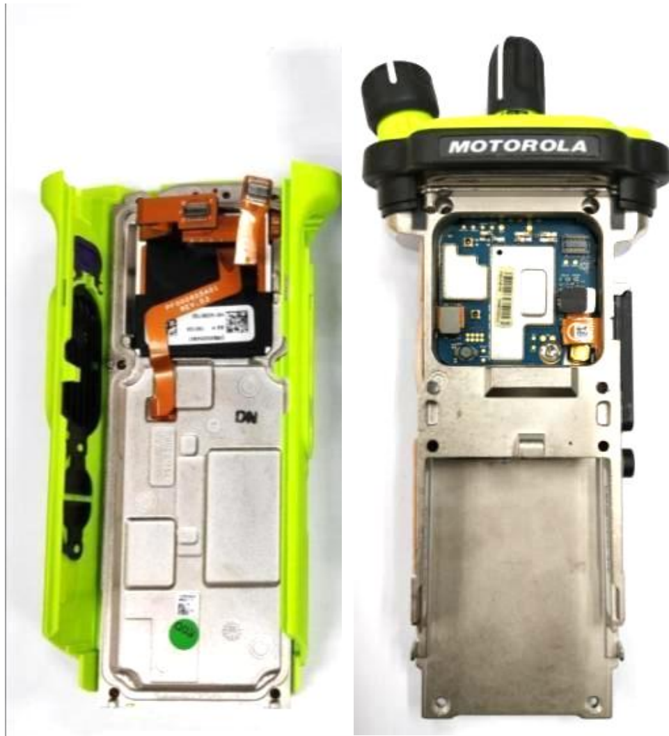
Expansion board with chassis and housing of APX8000HXE Model 2.5 (Back side)
