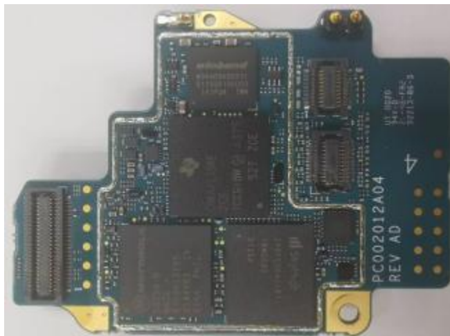
Vocon board without shields (Top) (APX8000H/8000HXE)
