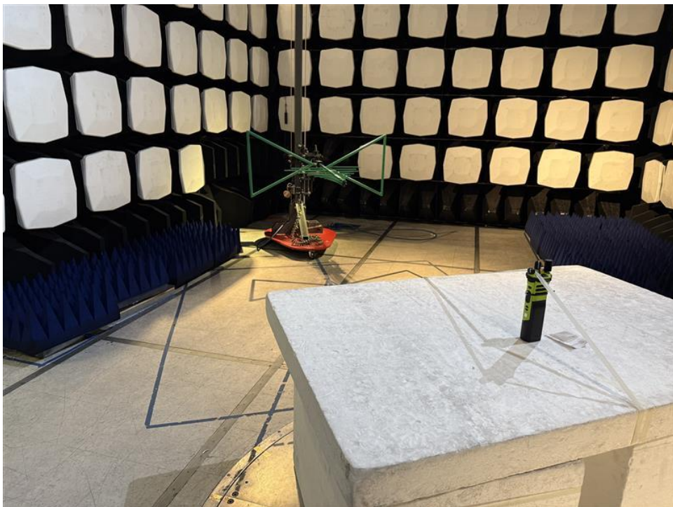
Figure A-4: Test Setup – Radiated Emissions < 1GHz
