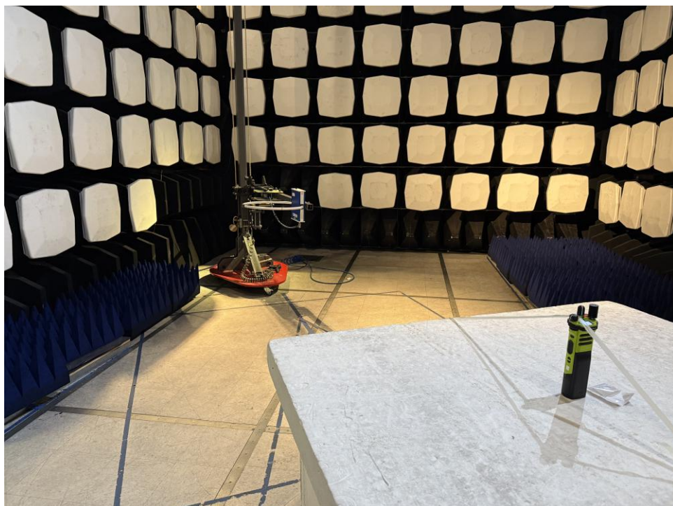
Figure A-2: Test Setup – Radiated Emissions < 30 MHz
