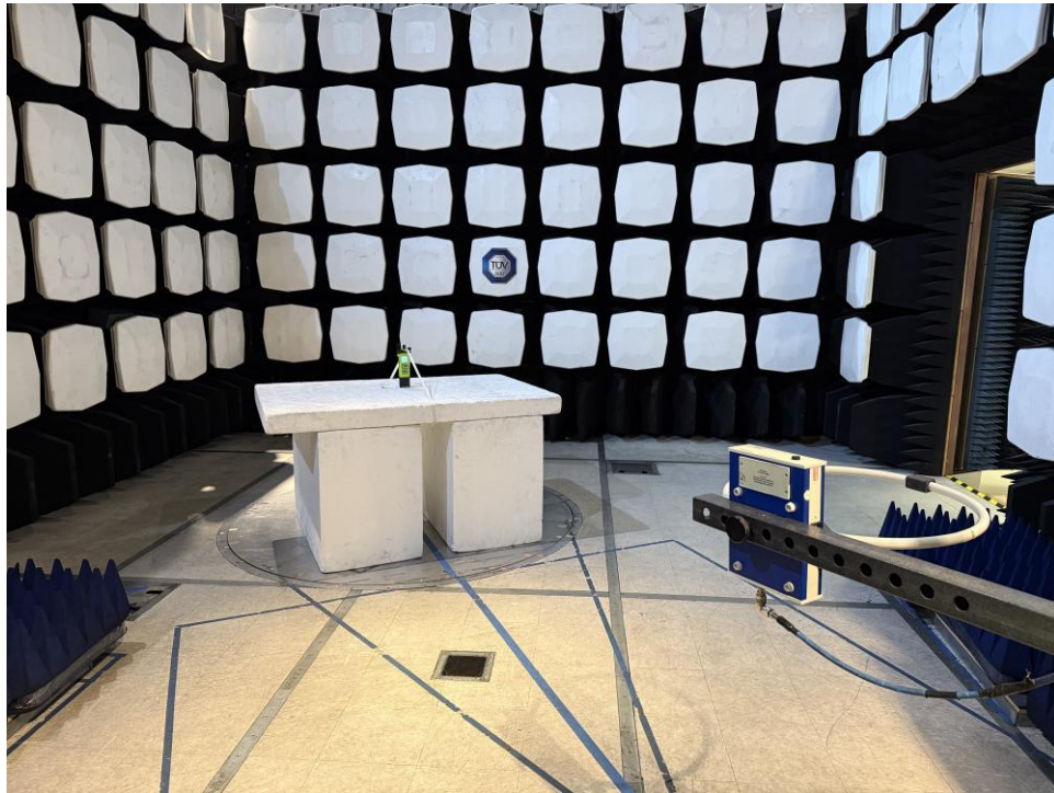
Figure A-1: Test Setup – Radiated Emissions <30 MHz
