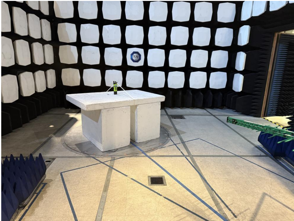
Figure A-3: Test Setup – Radiated Emissions < 1GHz
