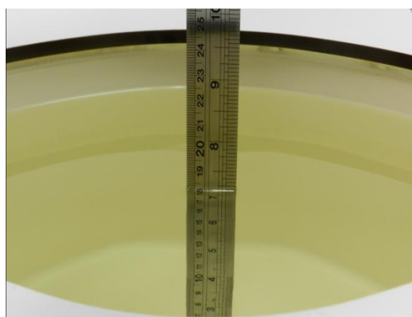
Fig 10.2 Photo of Liquid Height for Body SAR
