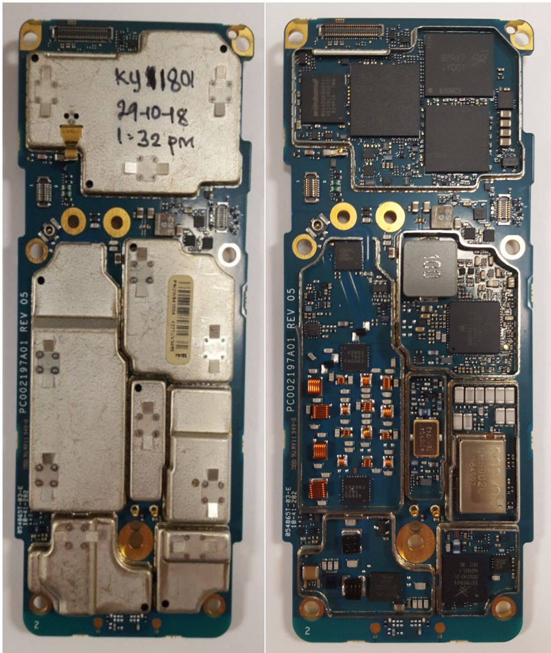
Exhibit 9A Main board with & without Shields (Top)
