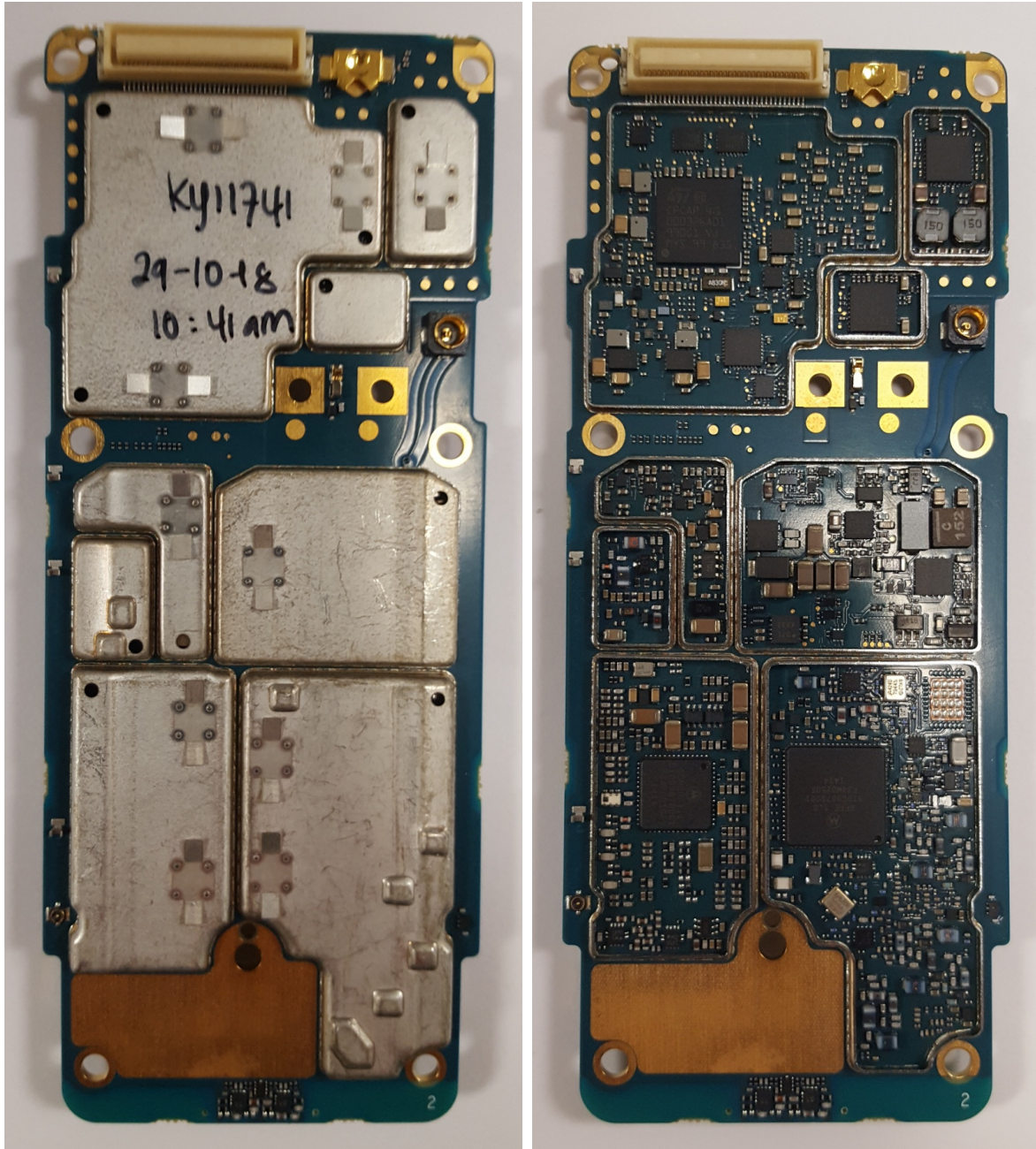
Exhibit 9B Main board with & without Shields (Bottom)
