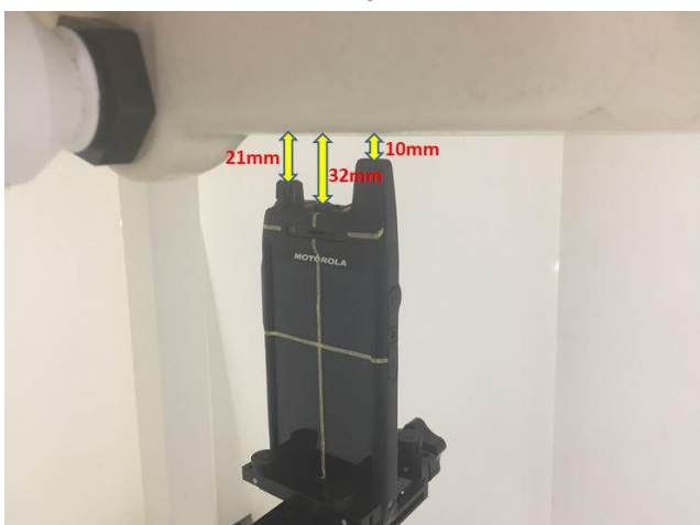
Top Side, Test Separation 10 mm
