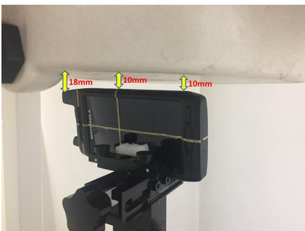
Right Side, Test Separation 10 mm
