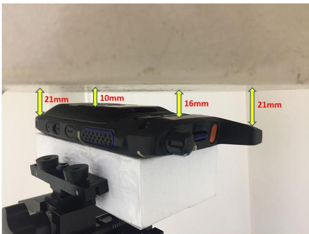
Back, Test Separation 10 mm
