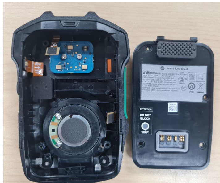
Overall Internal Assembly with housing (Back)
