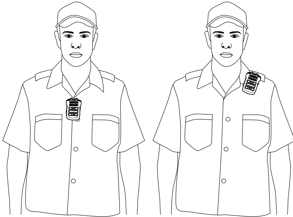
Figure 2: Recommended Wearing Positions—Using Tethering Kit Accessory with Lanyard
