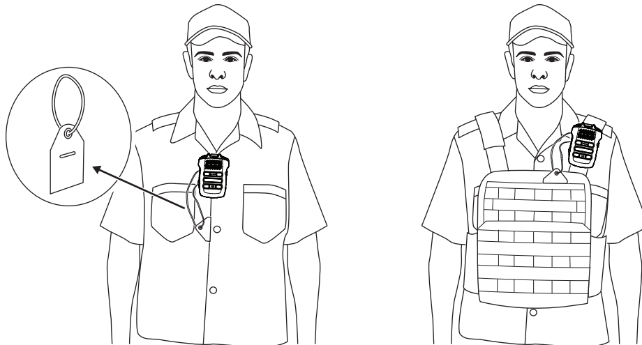
Figure 3: Recommended Wearing Positions—Using Tethering Kit Accessory with Velcro and Lanyard
