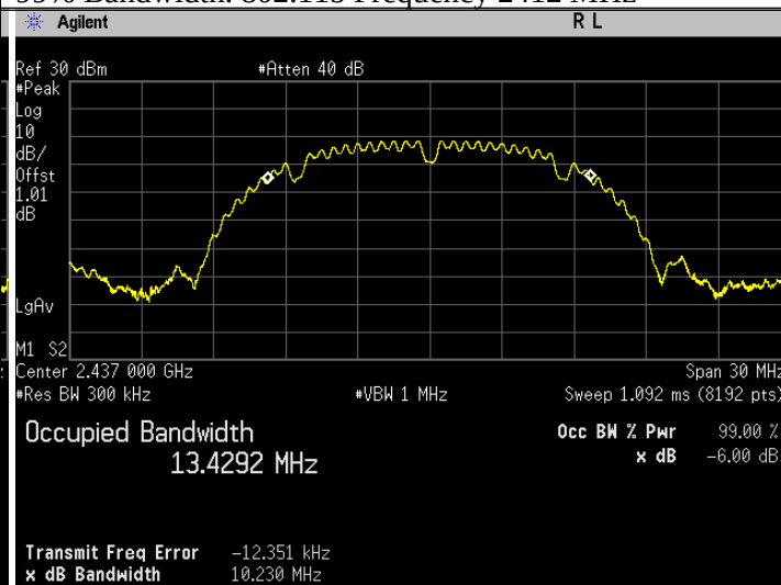
99% Bandwidth. 802.11b Frequency 2437 MHz
