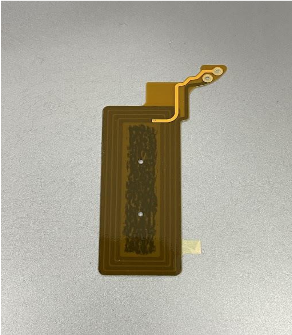
Figure 1: NFC Antenna Photo
