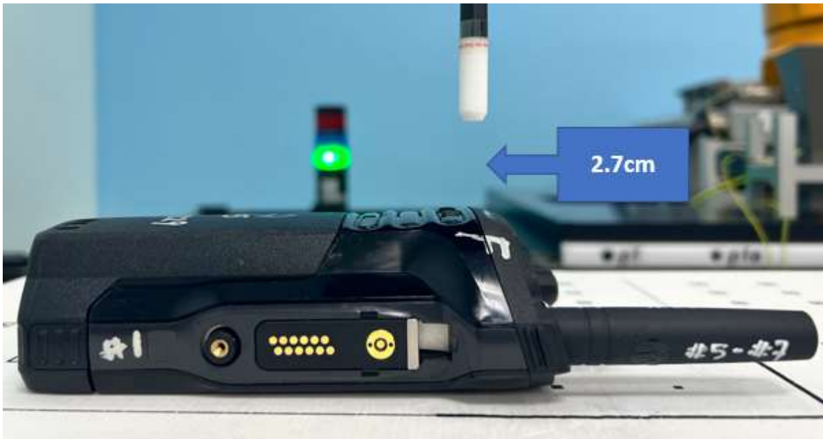
iPD for WiFi 6E DUT Scan Photo (Face Confiuration) DASY Sensor Surface Probe distance: 2mm Separation for Face configuration: 2.5cm
