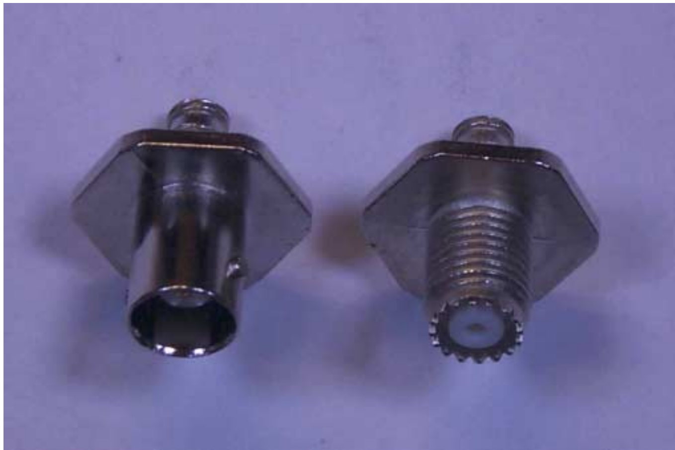
Figure 3-6: Close-up views of the BNC (left) and mini-UHF (right) antenna connectors.
