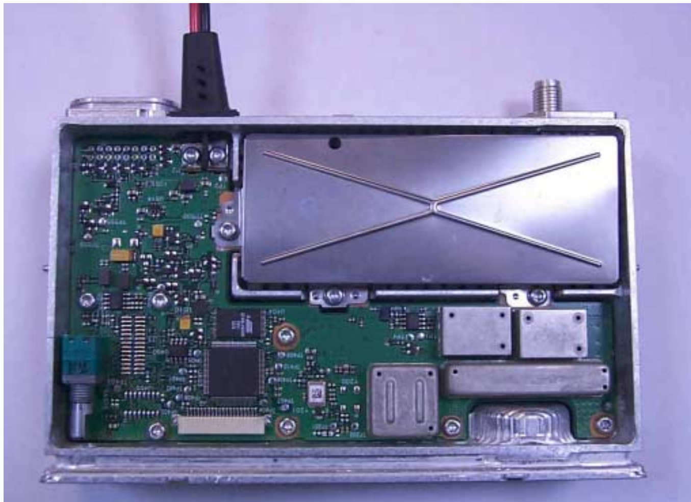
Figure 9-6: Top View of PCB placed in chassis with shield covering transmitter section.
