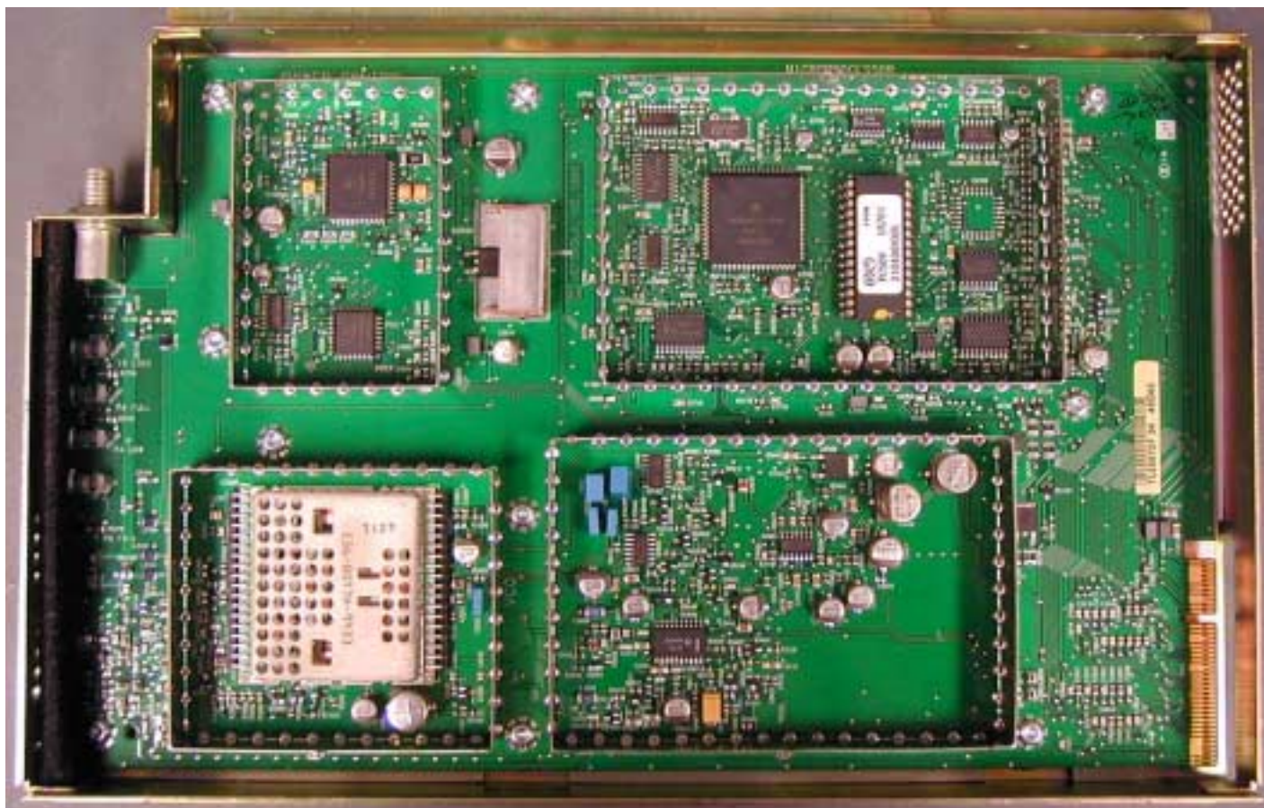
EXCITER MODULE WITH LID REMOVED
