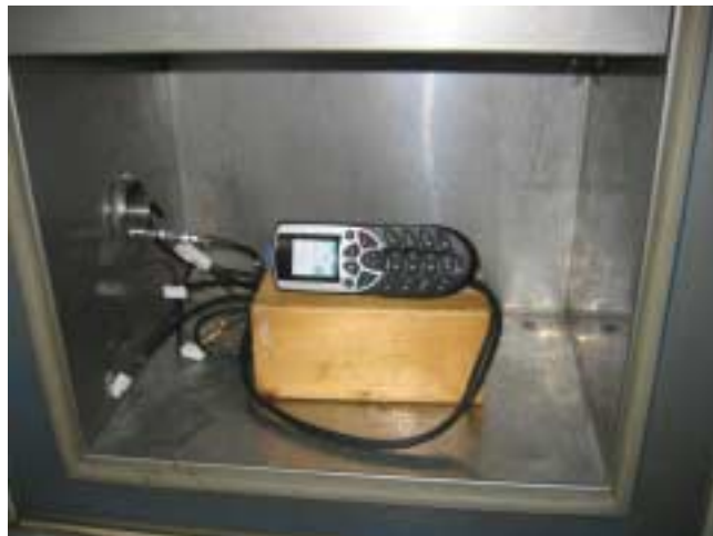
Photograph 7.6.1 Frequency stability test setup
