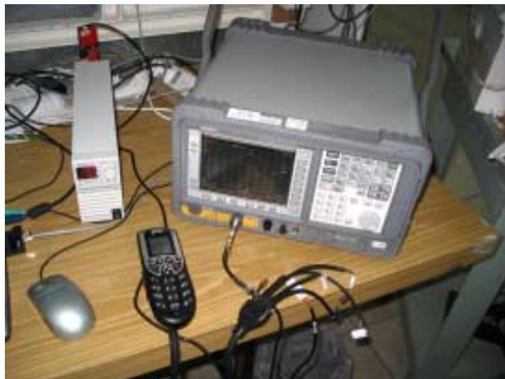
Photograph 7.5.1 Spurious emission test setup
