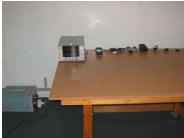
Photograph 8.1.1 Setup for conducted emission measurements
