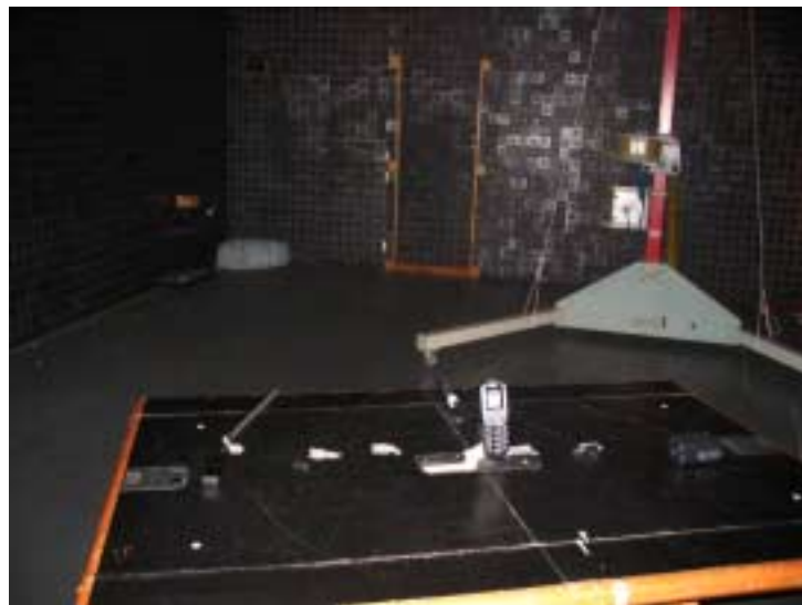
Photograph 8.2.1 Setup for preliminary radiated emission measurements
