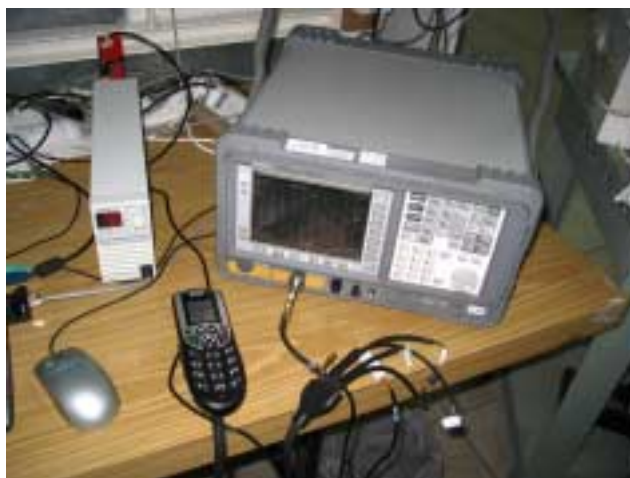
Photograph 7.2.1 Occupied bandwidth test setup
