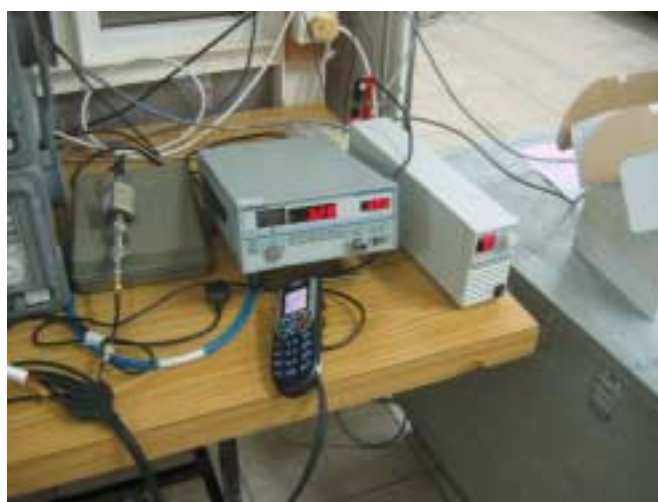
Photograph 7.1.1 Peak output power test setup
