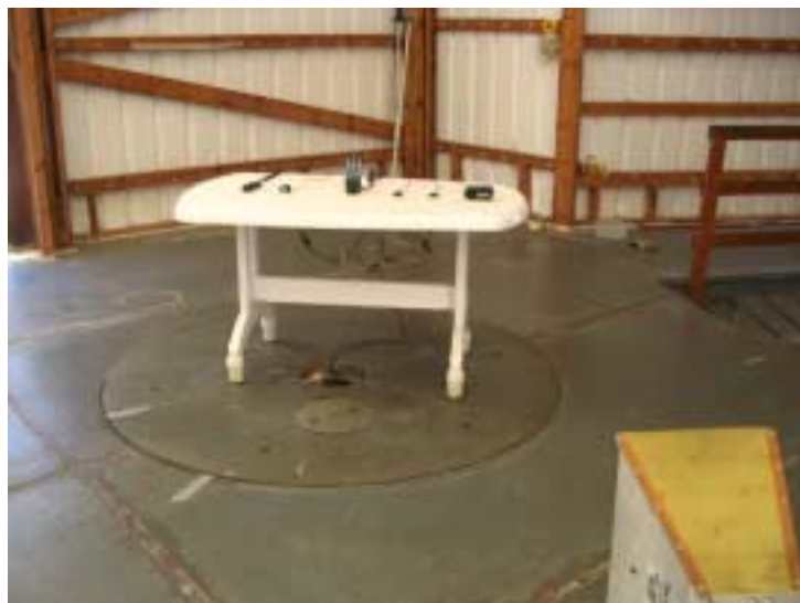
Photograph 7.4.2 Setup for spurious emission field strength measurements above 30 MHz
