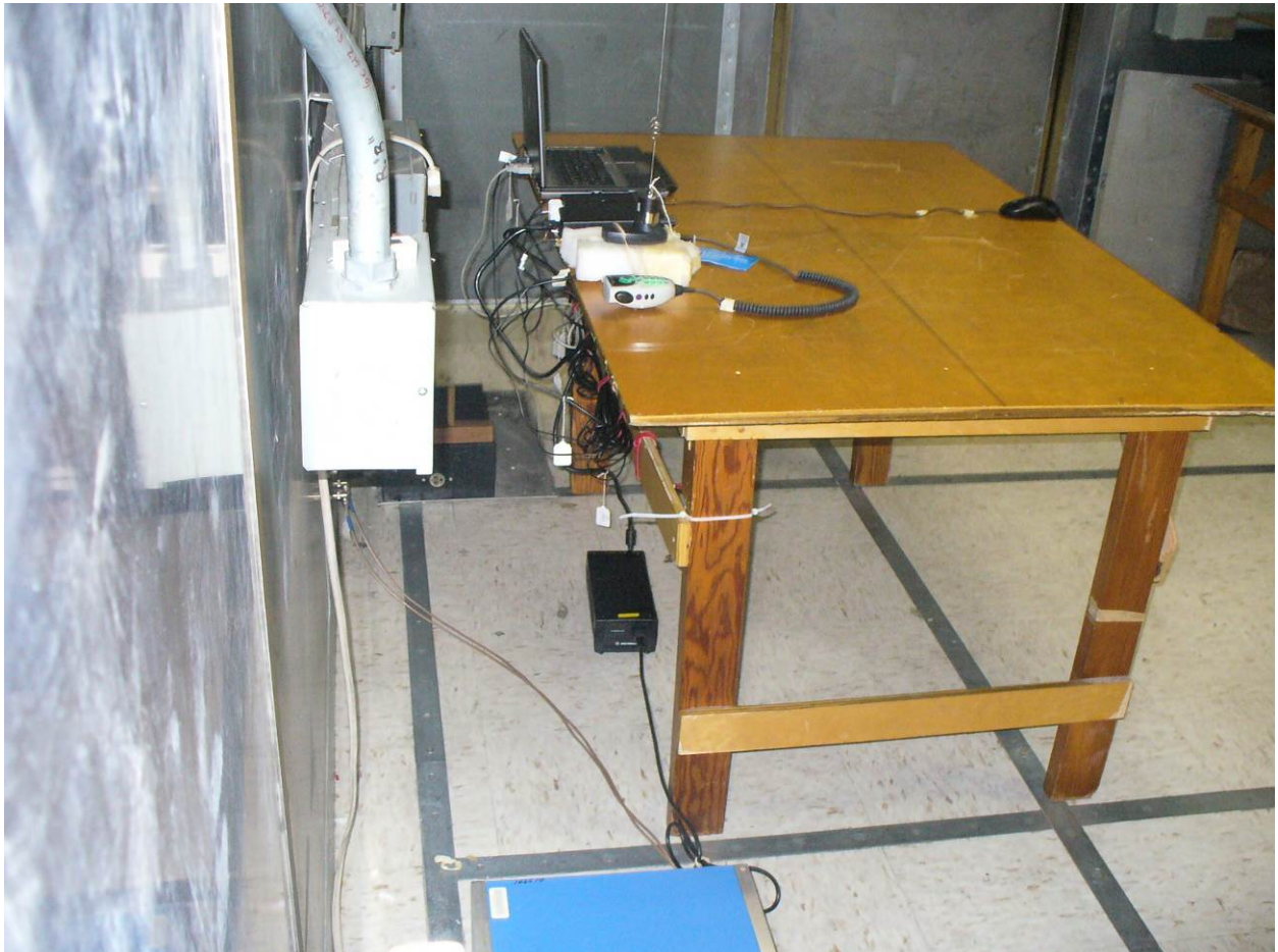
Figure 4: Power Line Conducted Emissions – Side View
