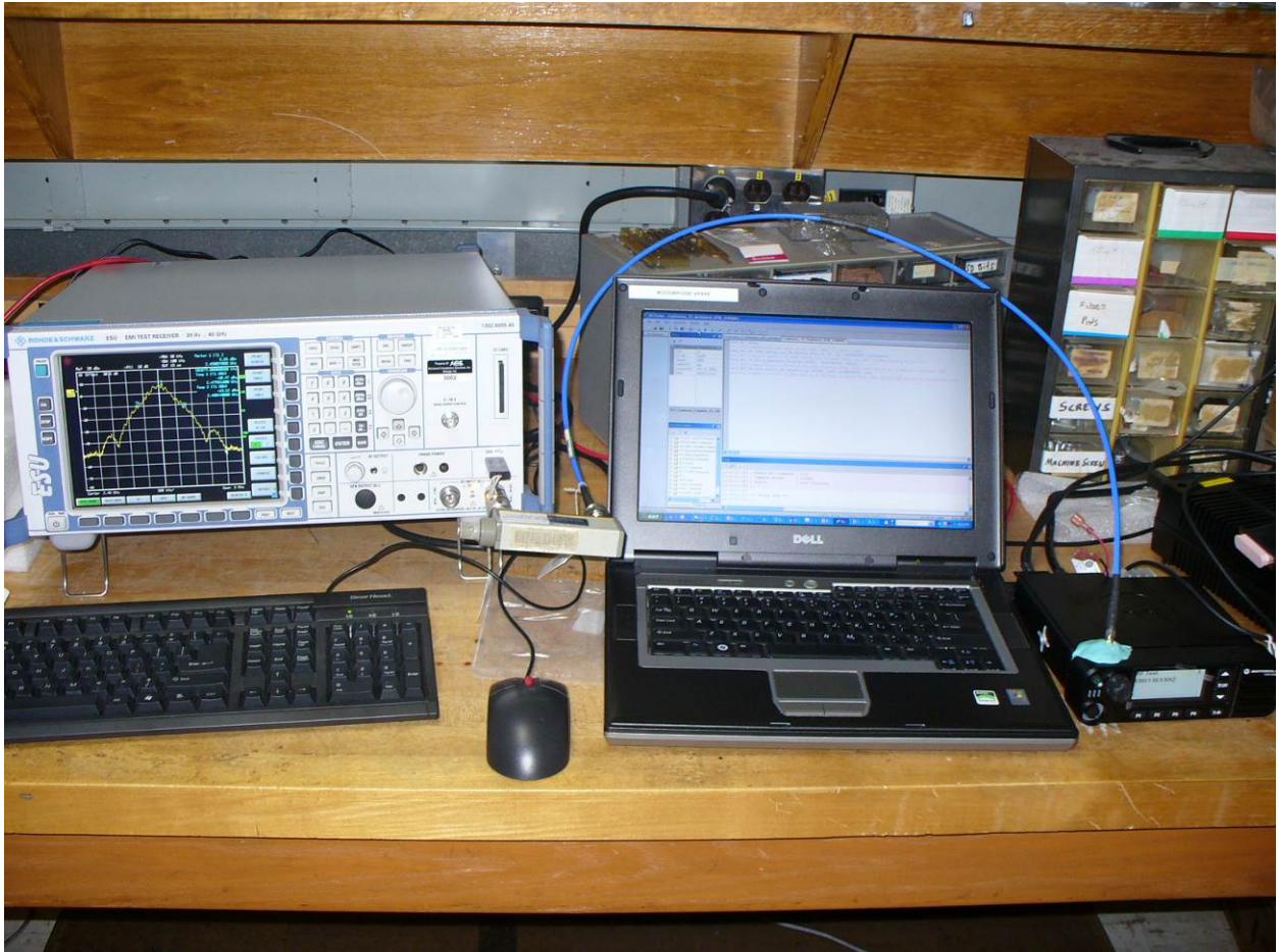
Figure 5: RF Conducted Emissions
