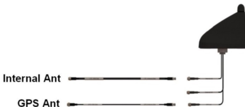
Figure 2-7 Diversity Antenna - Standard Configuration
