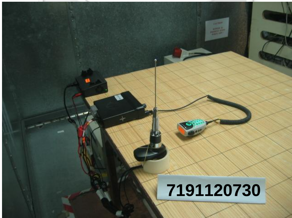
Conducted Emissions Test Setup (Rear View)
