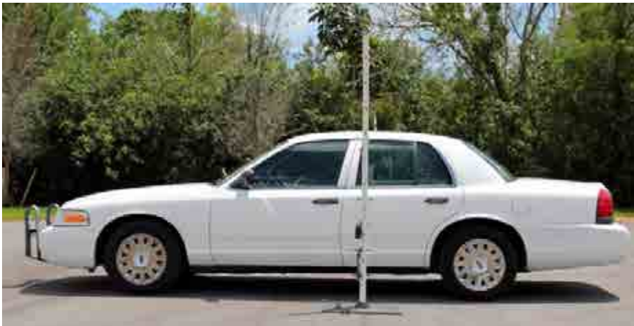
Test measurement setup for Bystander roof mount antenna
