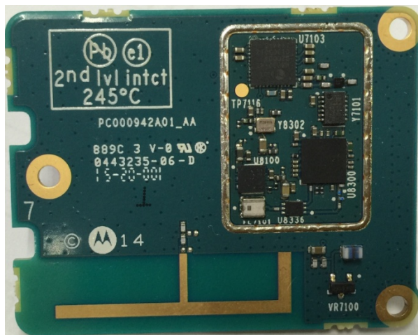
GPS/BT/Wifi board without shield (Bottom)
