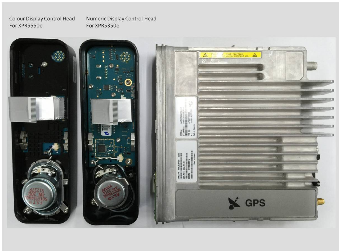
Chassis and control heads (Bottom)
