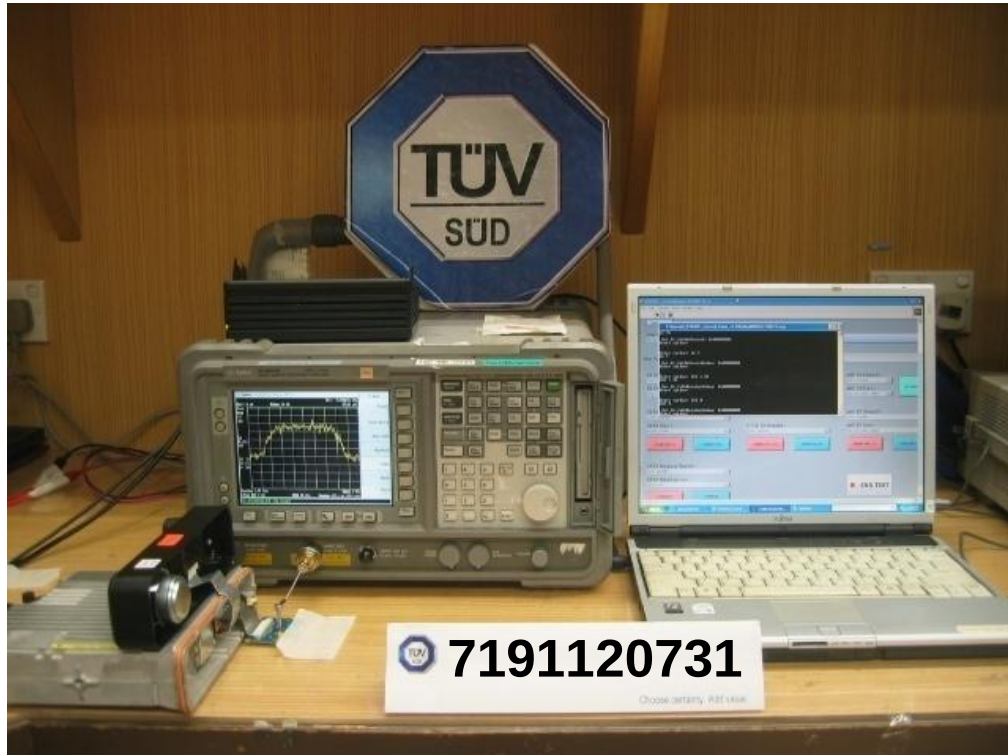
Carrier Frequency Separation Test Setup
