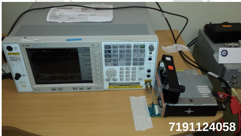
Average Frequency Dwell Time Test Setup
