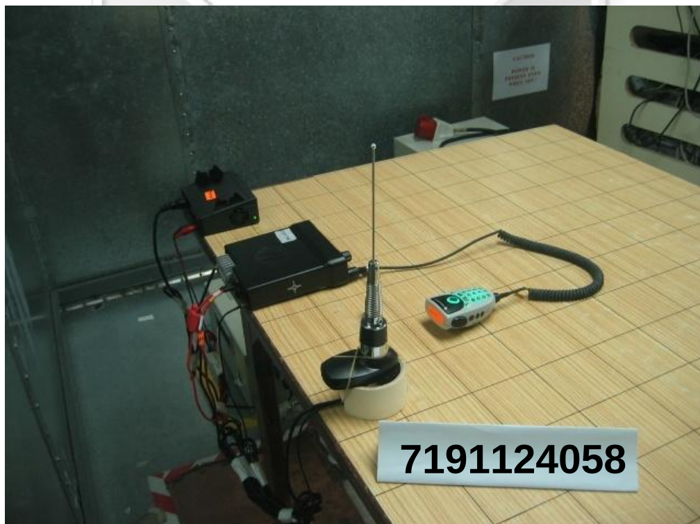
Conducted Emissions Test Setup (Rear View)
