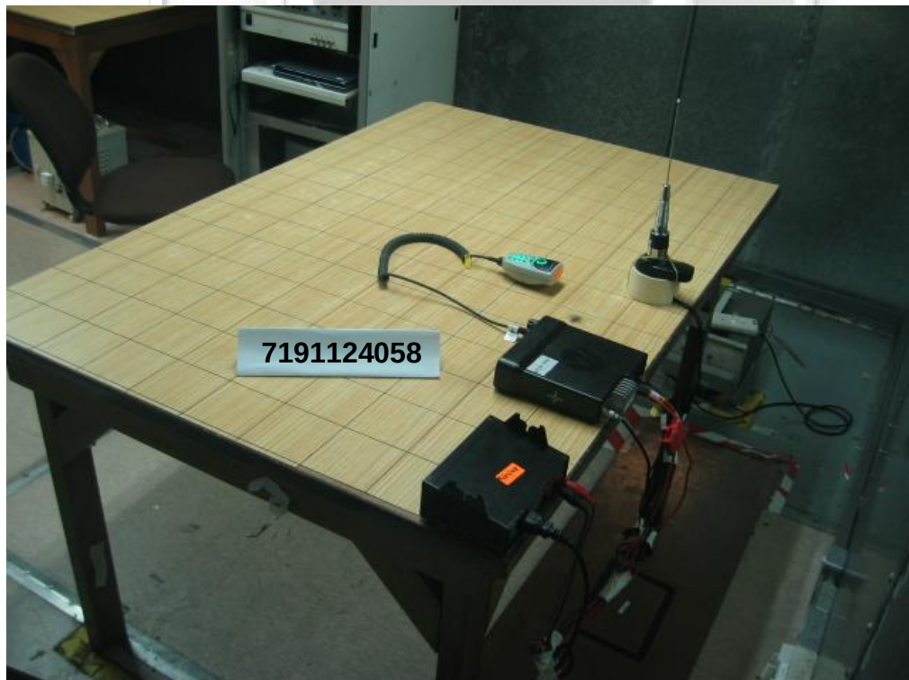
Conducted Emissions Test Setup (Rear View)
