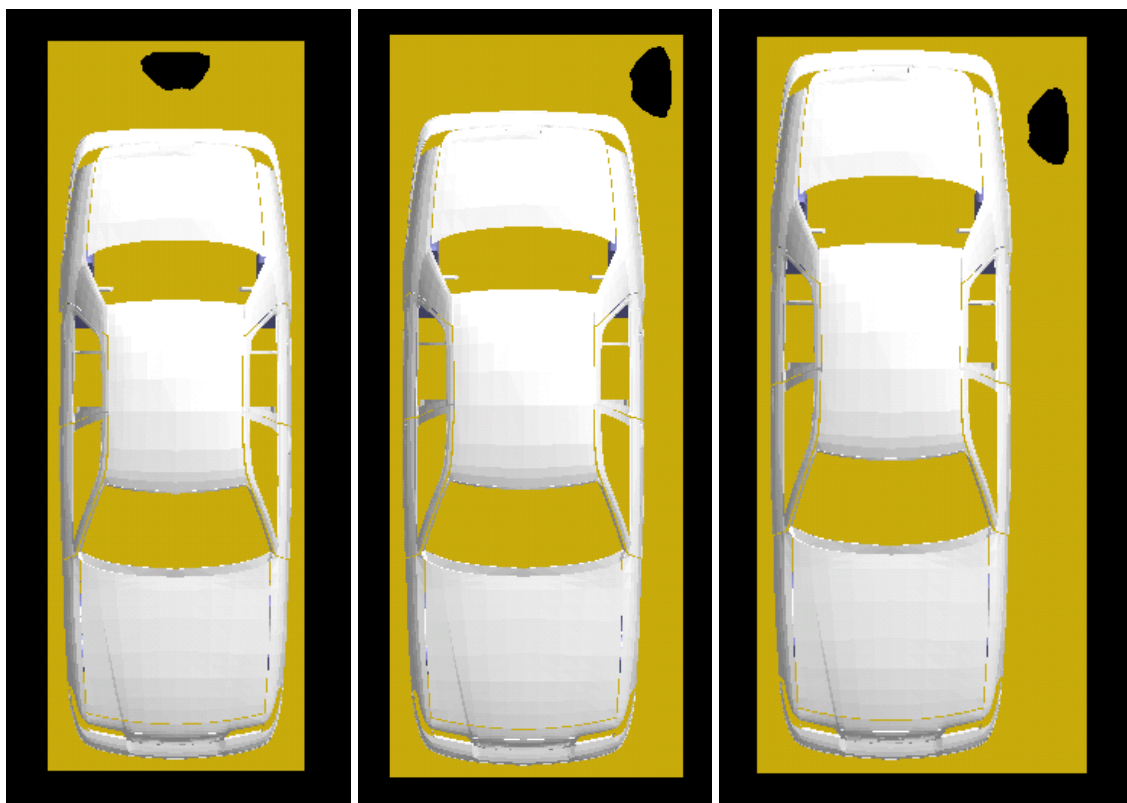
Figure 3: Top view of bystander exposure model four different locations relative to the vehicle model that replicate the measurement conditions.
