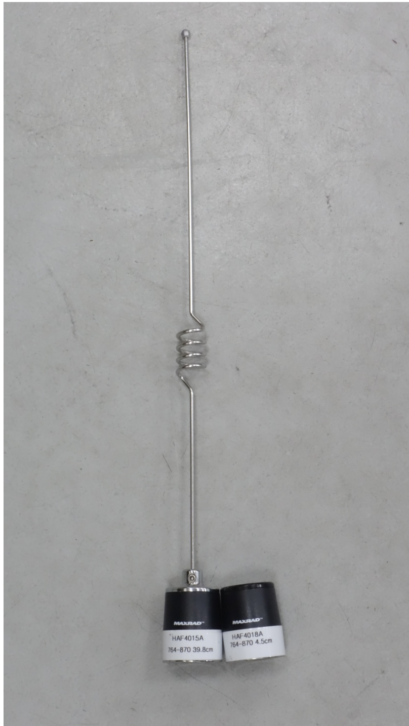
7/800 Antenna kit numbers, from left to right; AN000197A10 (HAF4015A) and AN000197A11 (HAF4018A)
