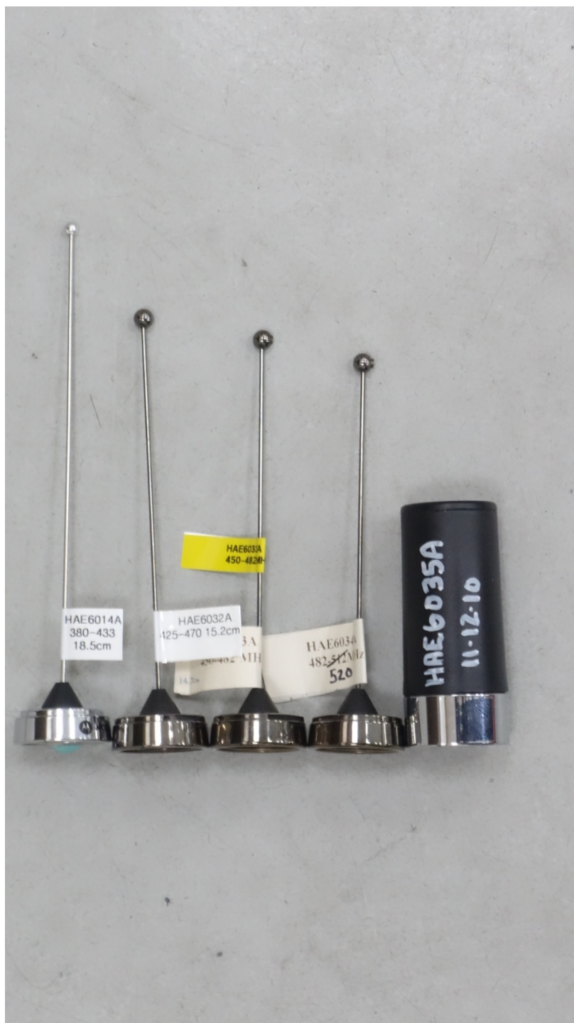
UHF Antenna kit numbers, from left to right; AN000197A05 (HAE6014A), AN000197A06 (HAE6032A), AN000197A07 (HAE6033A), AN000197A08 (HAE6034A) and AN000197A09 (HAD4026A)
