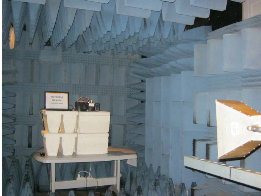
Figure 7. Radiated Emission Test, 1000-2000MHz
