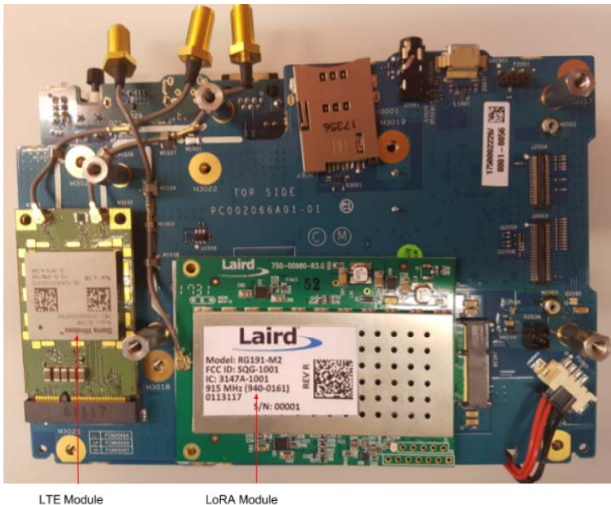
MC-EDGE Piggy Board Top View (APX4000 UHF1 Removed, with LORA and LTE) Without Front Panel
