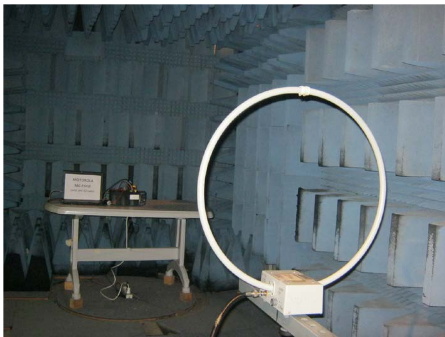
Figure 4. Radiated Emission Test, 0.009-30MHz
