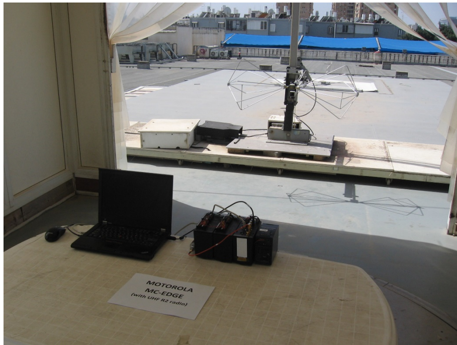
Figure 5. Radiated Emission Test, 30-200MHz
