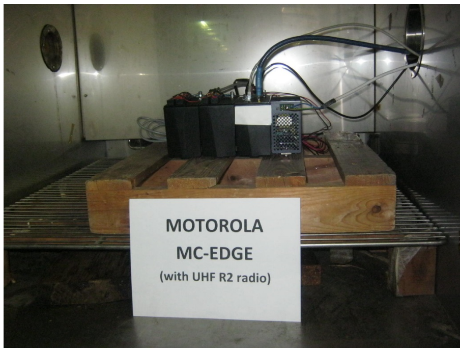
Figure 8. Frequency Stability Test
