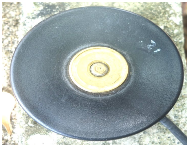
Magnetic mount base (top and side view)
