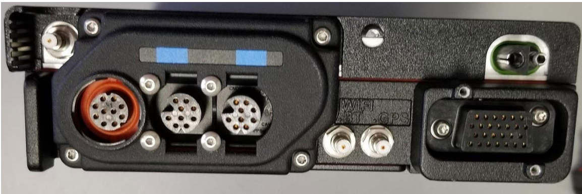
APX 8500 BACK VIEW (TIB added for Control Head interface)
