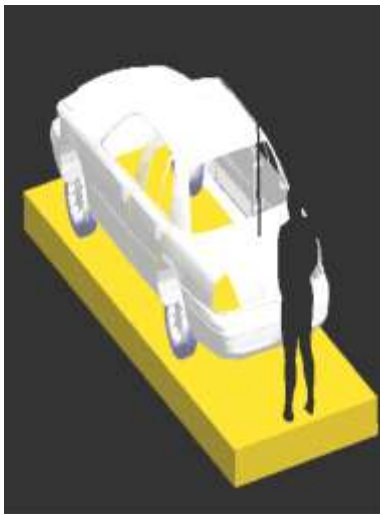
Figure 4: Bystander model exposed to a trunk-mount antenna: XFDTD™ geometry.
