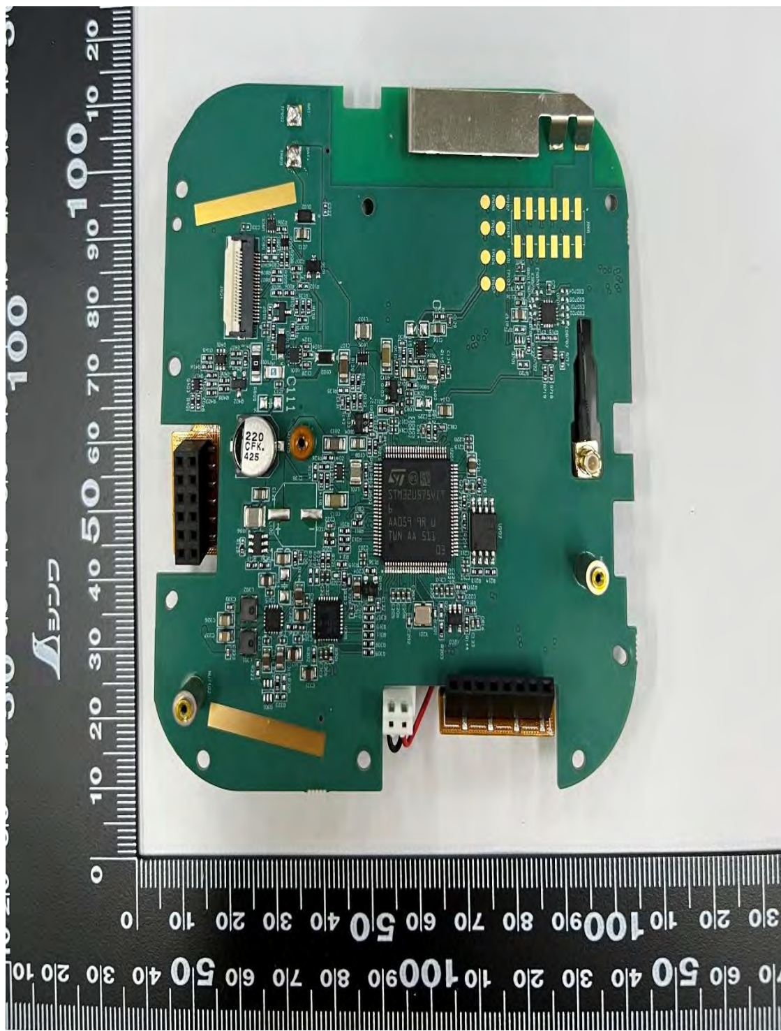
Main Board (Bottom) - CBS101NBKLBA (CB900D) CB900D 1-Way Call Box
