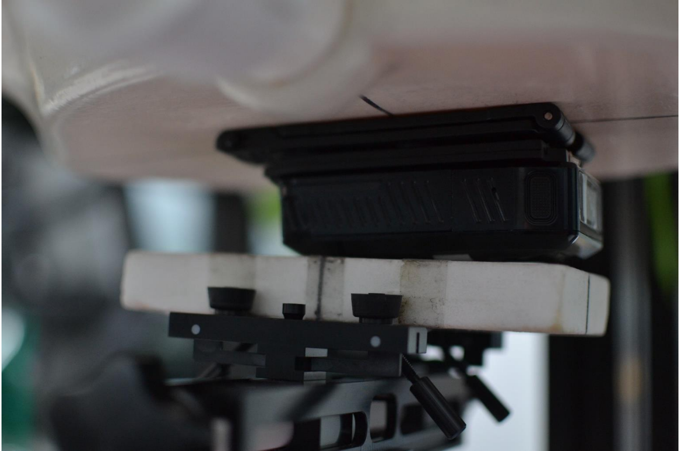
SAR Test Setup Photo 3 – Mount WGA00668, Back Side at 0mm
