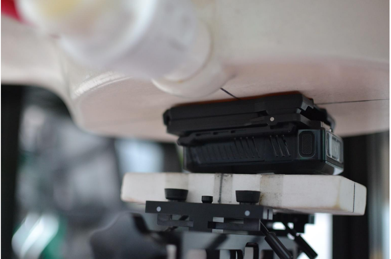
SAR Test Setup Photo 5 – Mount WGP03085, Back Side at 0mm
