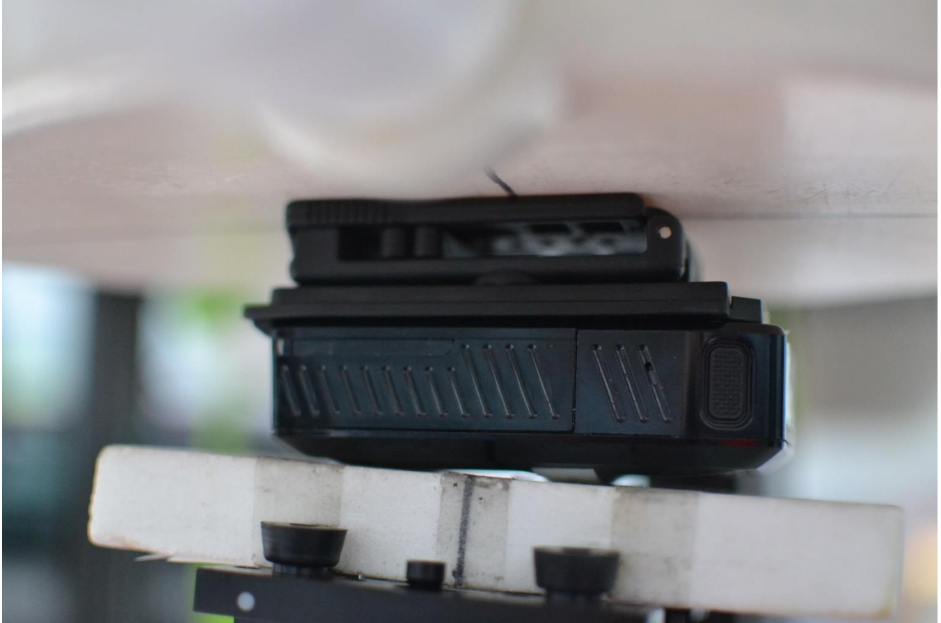
SAR Test Setup Photo 4 – Mount WGA00669, Back Side at 0mm
