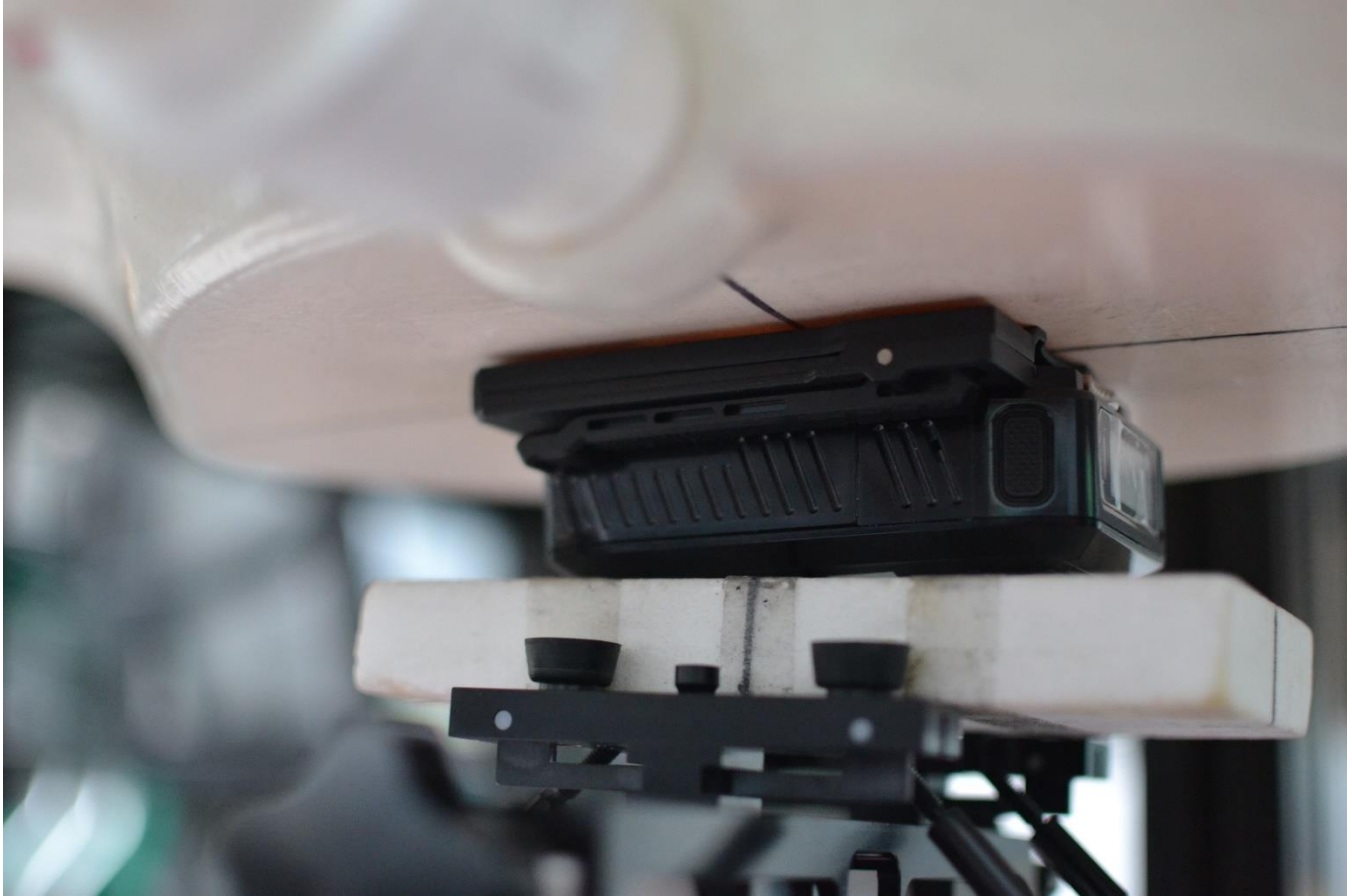
SAR Test Setup Photo 6 – Mount WGP02798C, Back Side at 0mm
