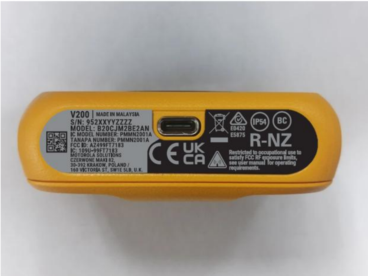
Figure 4: FCC/IC Label Location for V200 (Yellow)
