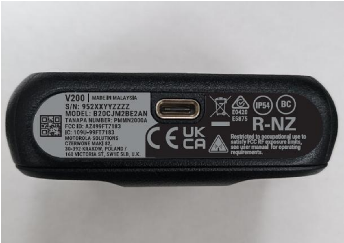
Figure 3: FCC/IC Label Location for V200 (Black)
