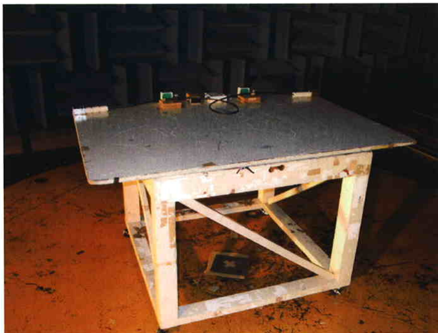
Photo 7.1a Setup with the Maximized RFI Field Strength Emission Level (Semi Anechoic Chamber)
