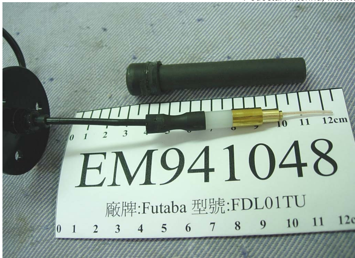
Figure 13 Pedestal Antenna, Internal View
