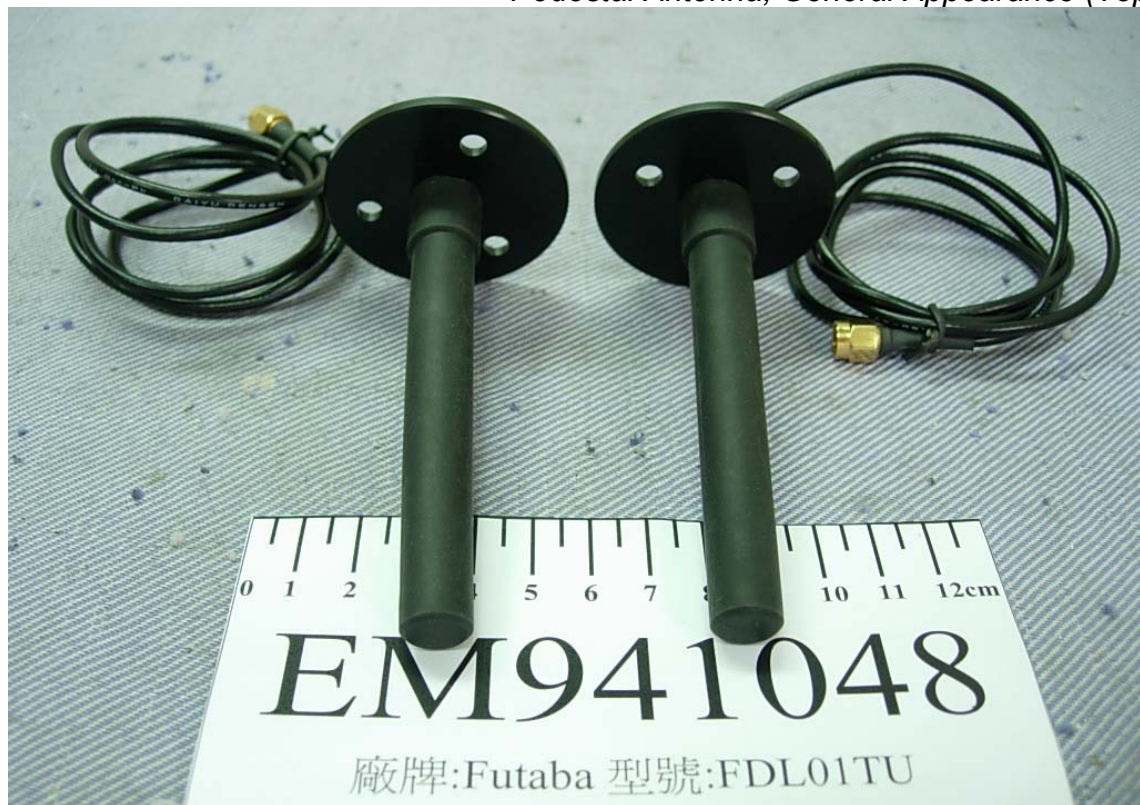
Figure 11 Pedestal Antenna, General Appearance (Top View)
