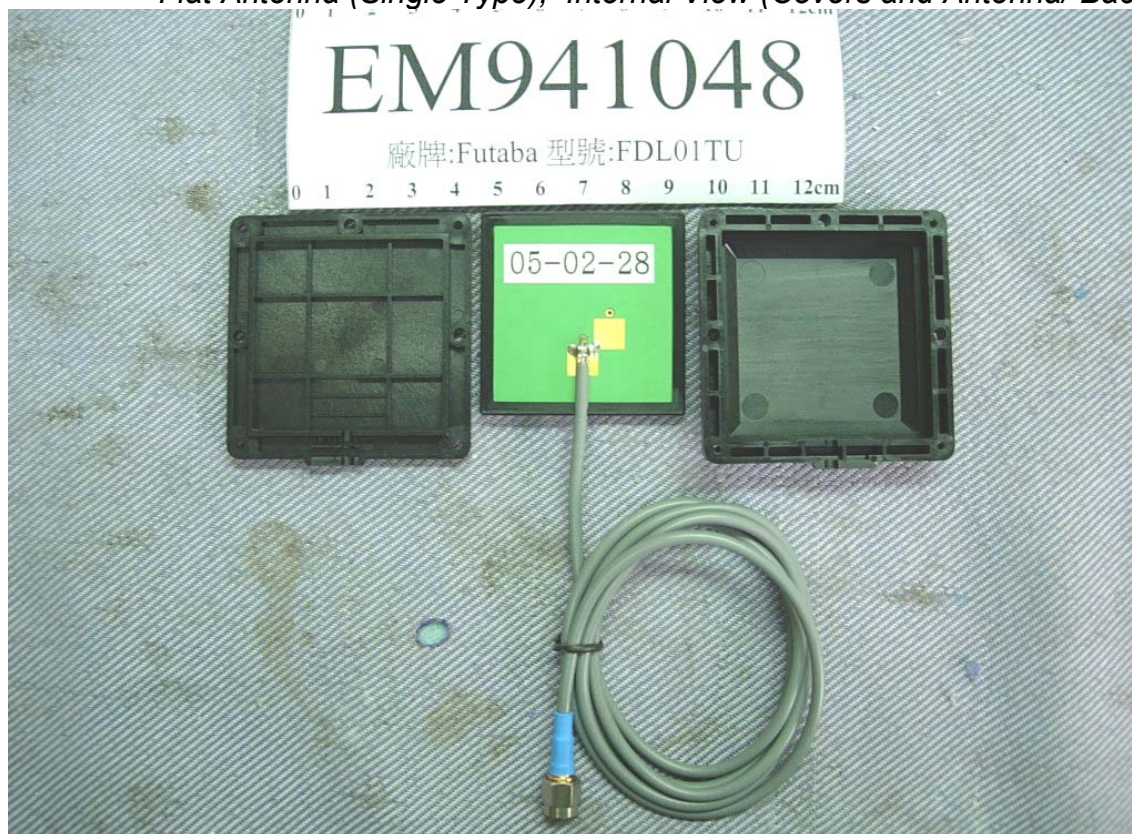
Figure 16 Flat Antenna (Single Type), Internal View (Covers and Antenna/ Back View)
