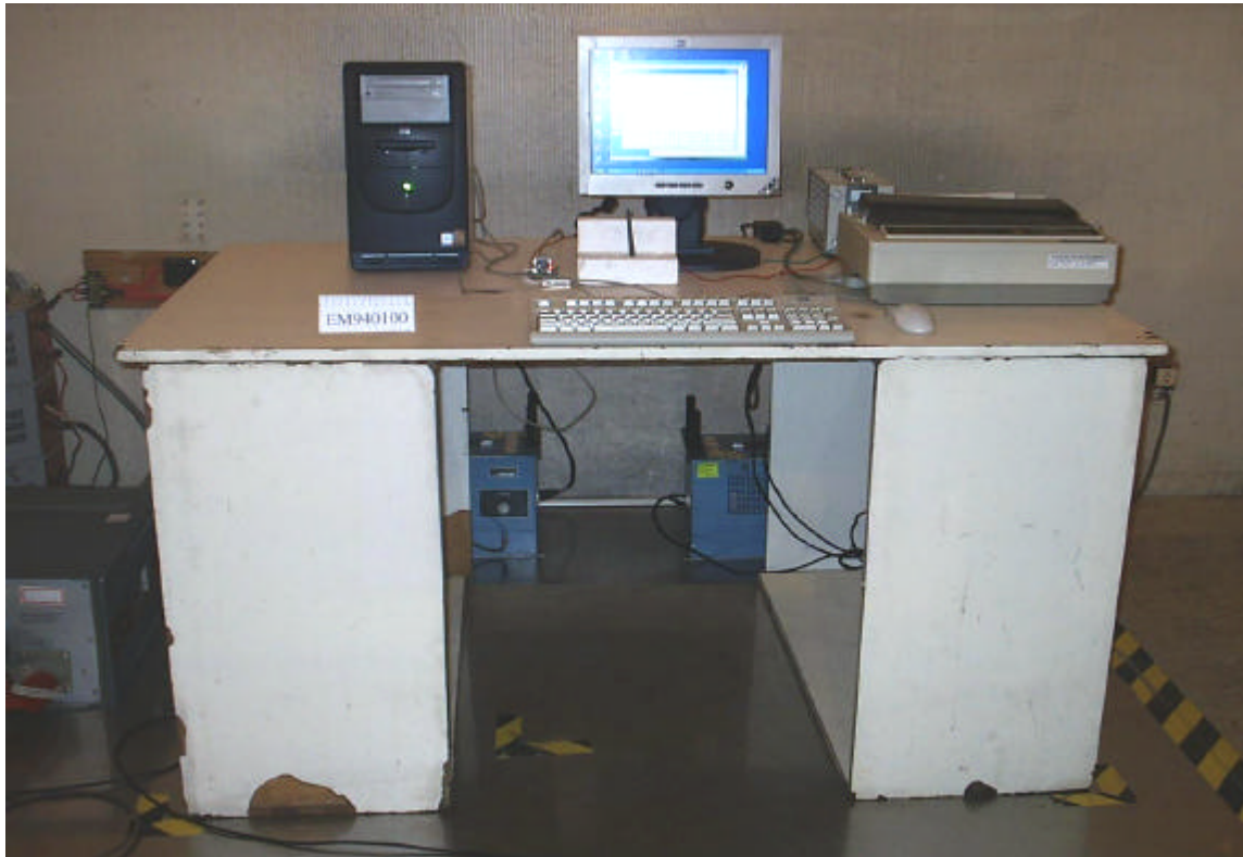
FRONT VIEW OF CONDUCTED MEASUREMENT
