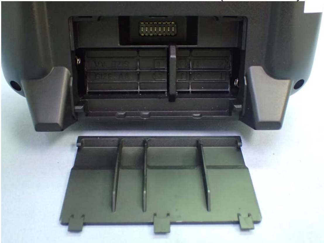
Figure 3 Internal View (Removed Battery Cover)
