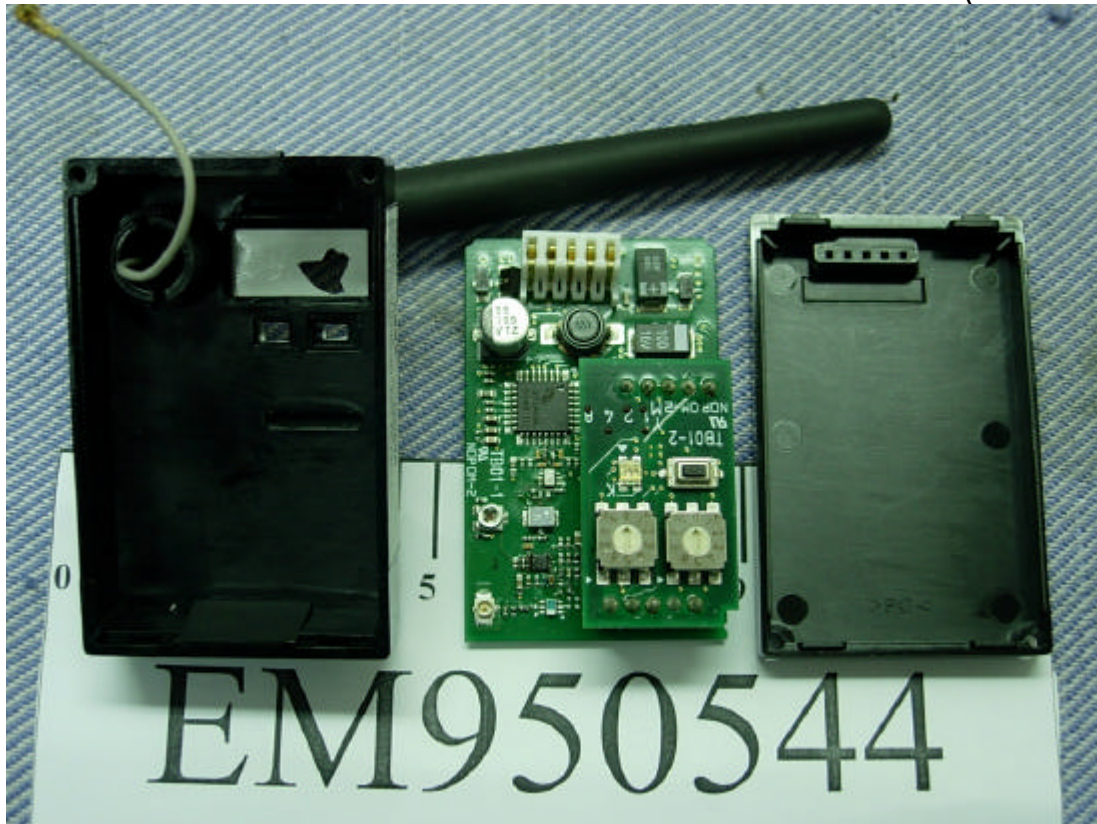
Figure 3 Internal View(Removed Cover)
