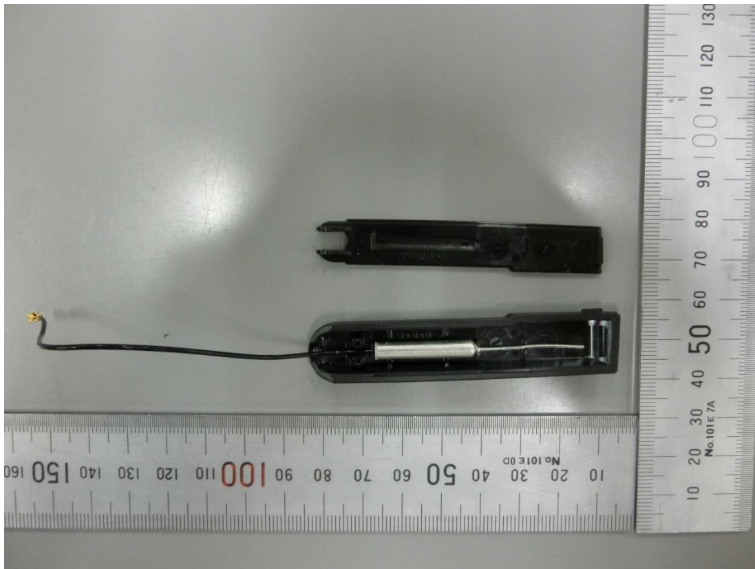
Figure 31 Internal View of Antenna
