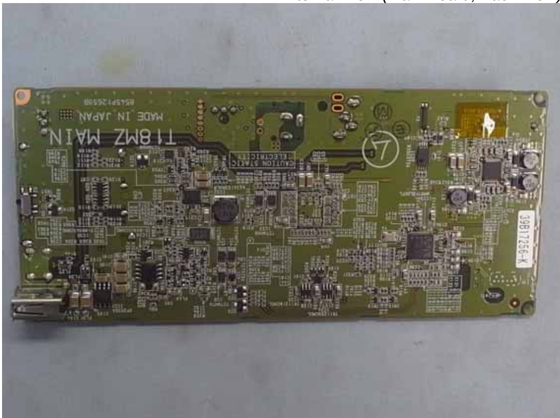
Figure 28 Internal View (Main Board, Back View)
