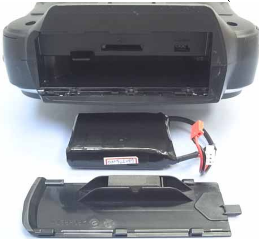
Figure 3 Internal View (Removed Battery Cover)
