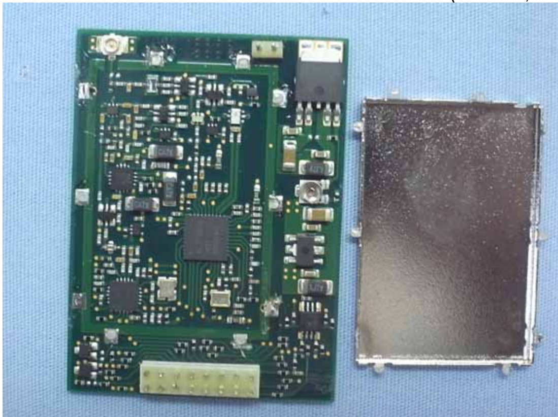
Figure 10 Internal View (RF Board, Front View)
