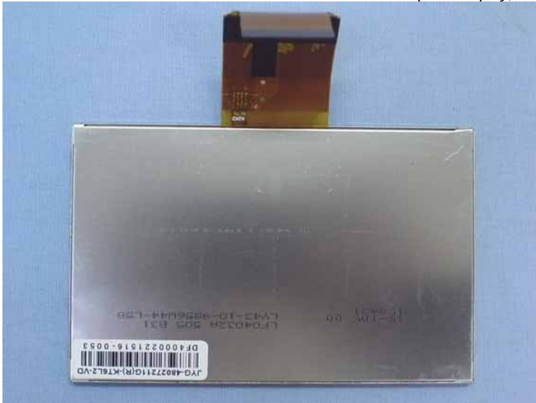
Figure 19 Internal View (LCD Display, Back View)
