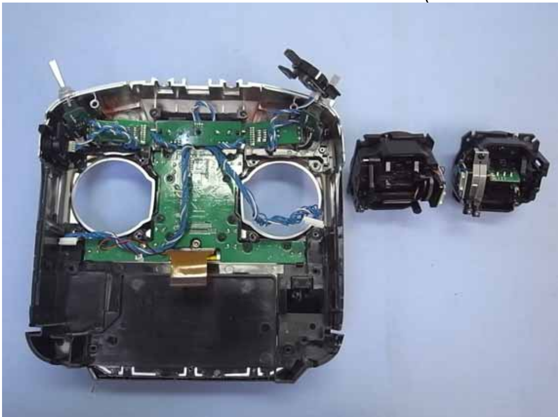
Figure 12 Internal View (Removed Control Boards)
