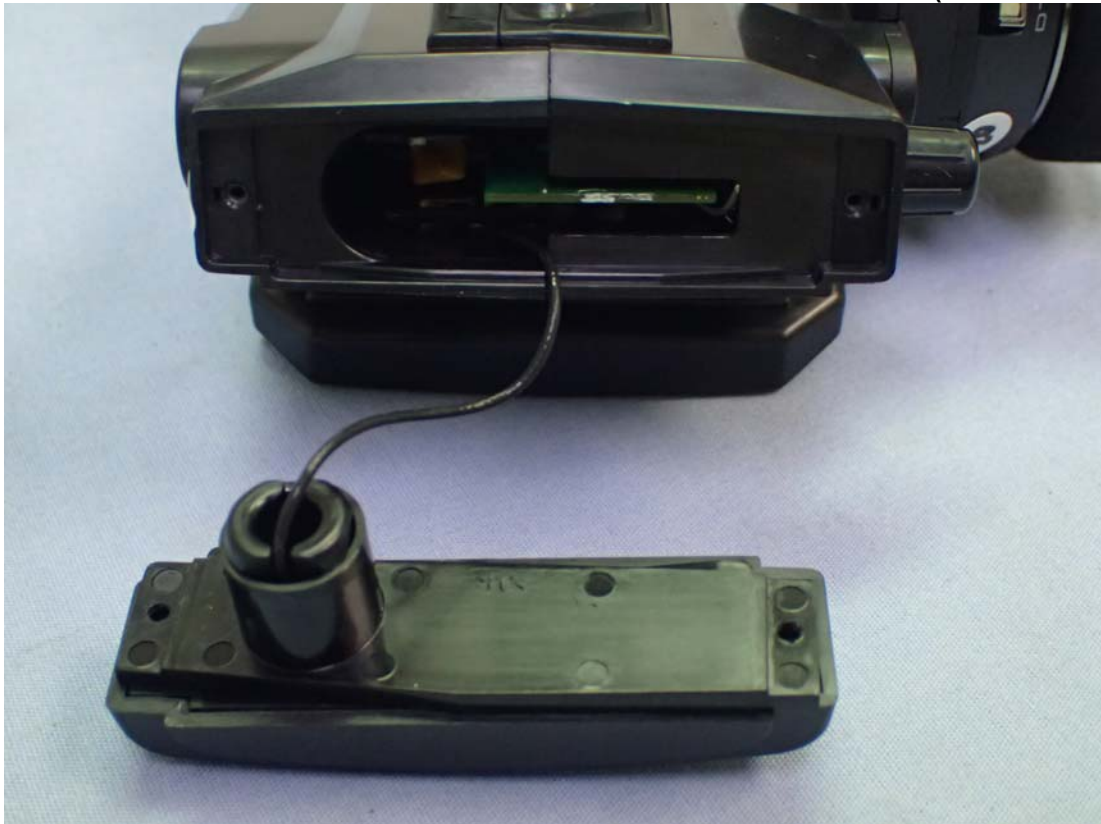
Figure 7 Internal View (Removed RF ANT)
