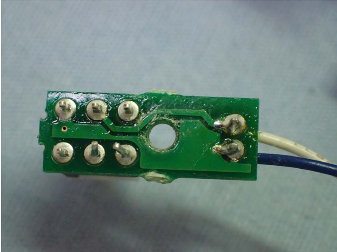
Figure 21 Internal View (TC11A-6 Board, Back View)
