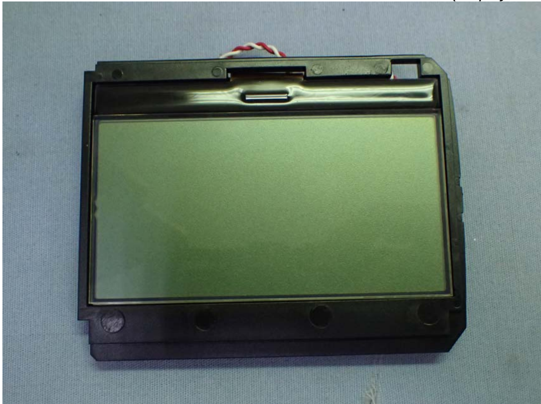
Figure 13 Internal View (Display, Front View)
